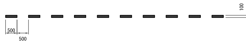
SIDE LINE ② (SHORT BROKEN WHITE) S=1:100
