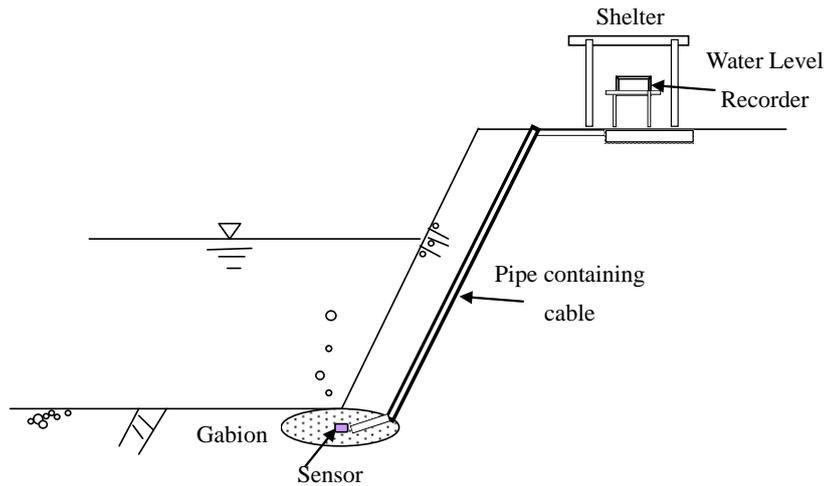
**Figure 1-2 Image of Water level Monitoring Station**
