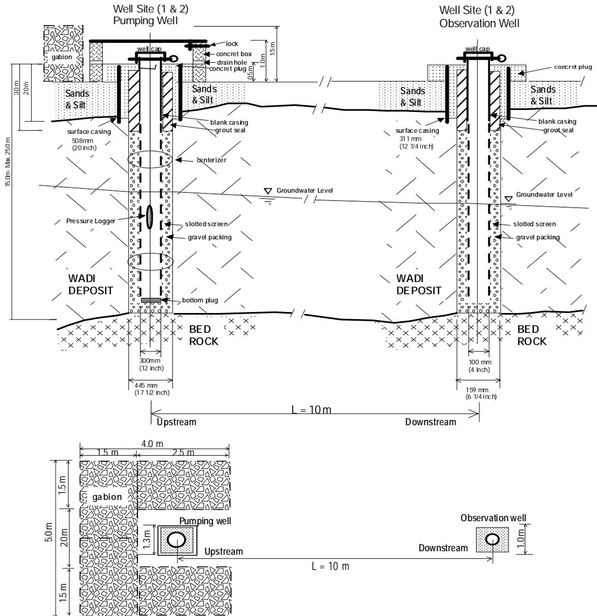
Figure 1-6 Typical Layout of Well Monitoring
