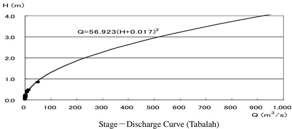
**Figure 2-2(1) Cross Section and Stage-Discharge Curve (Hirjab, Tabalah)**
