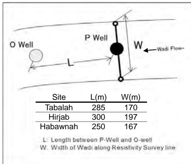
Figure 2-14 Layout of Base Flow Measurement Site
