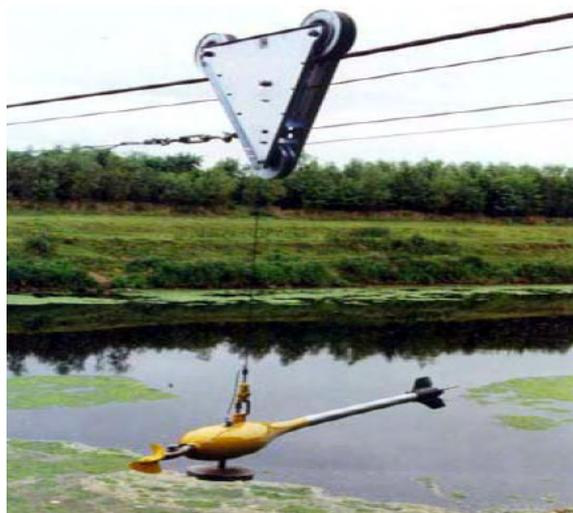
**Figure 1-5 Cableway Gauging System**
