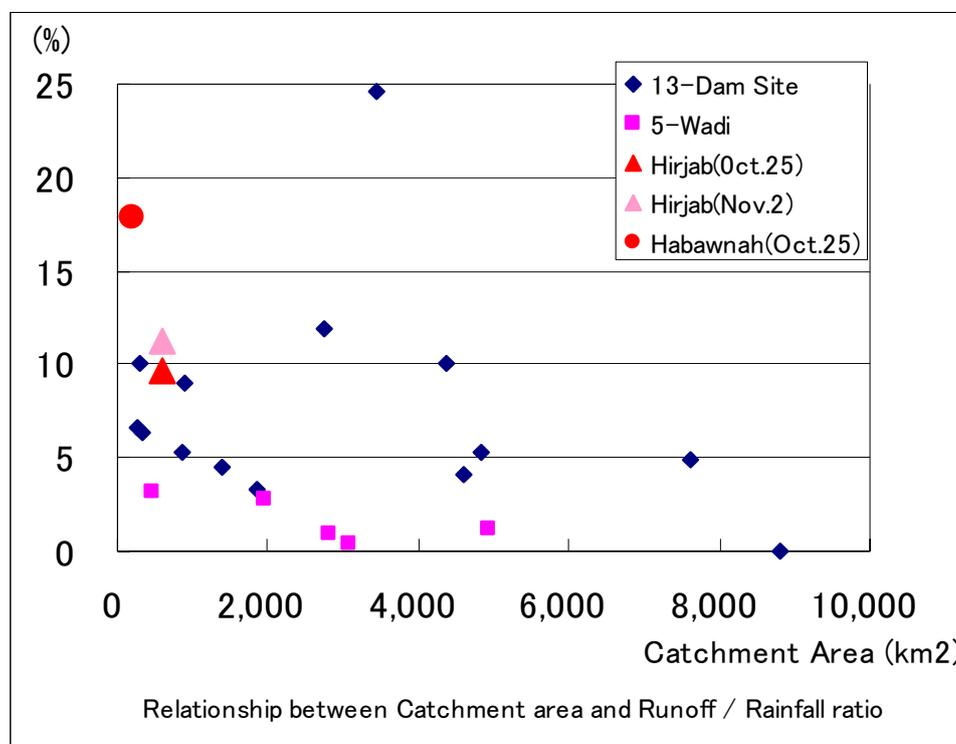
**Figure 2-6 Observed Flow Ratio**
