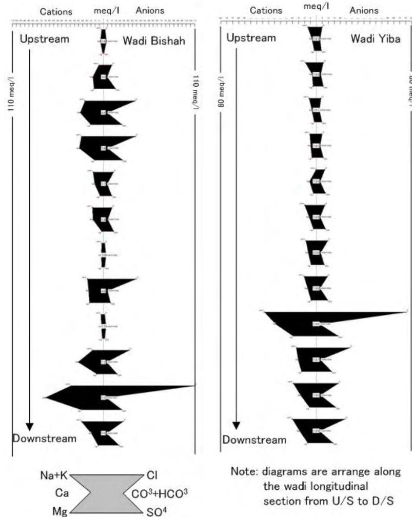
Figure 2-12 Changes of Water Quality in Wadi (Stiff Diagram)
