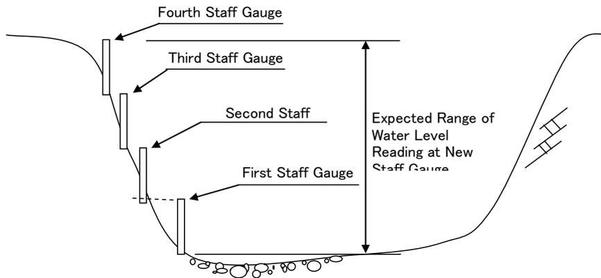
**Figure 1-3 Schematic Diagram of New Staff Gauge Installation**
