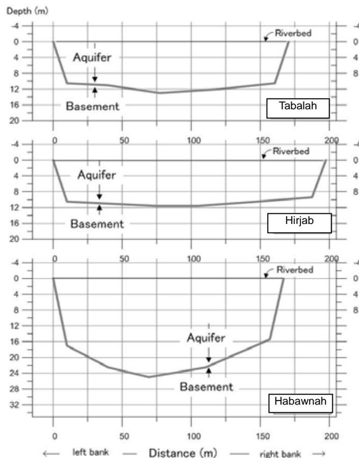
Figure 2-16 Thickness of Aquifer
