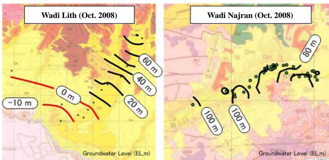
Figure 2-9 Groundwater Contour(Wadi Al Lith, Wadi Najran)
