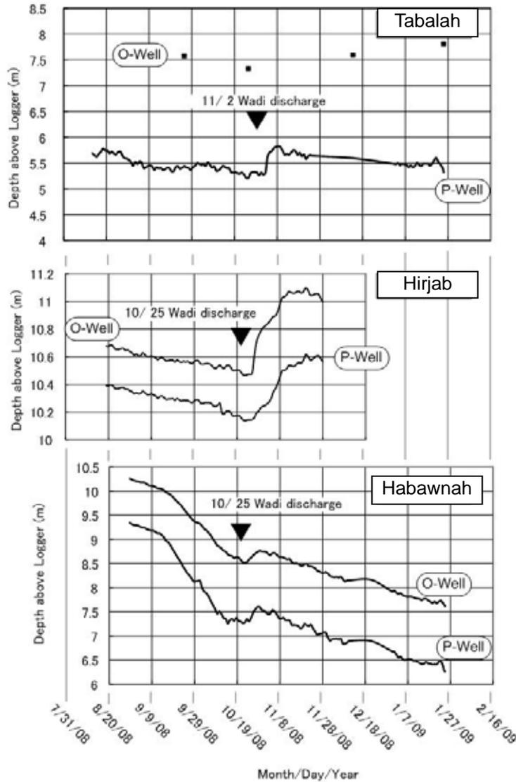
Figure 2-18 Groundwater Changes of Base Flow Stations
