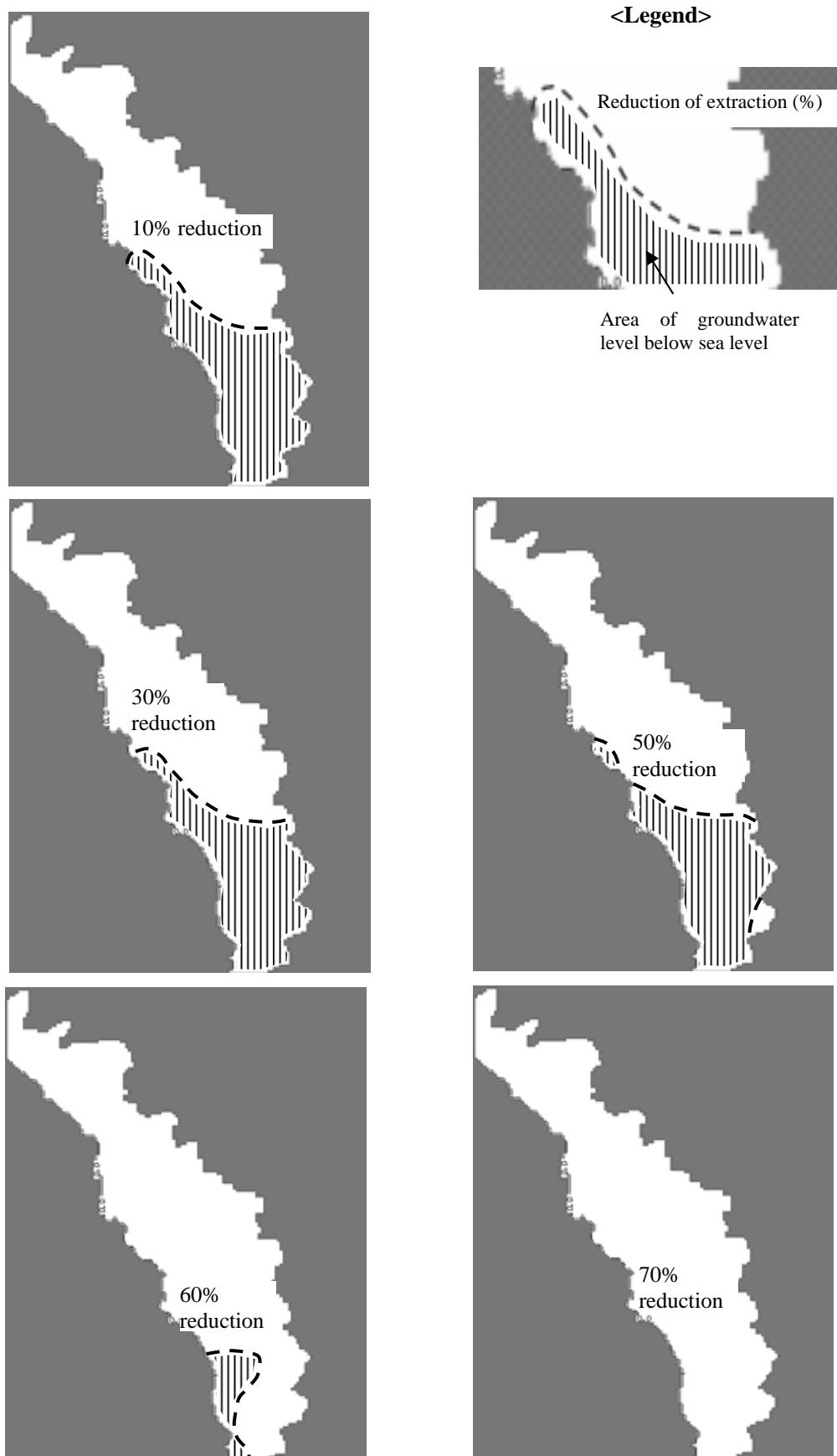
Figure 2-2 Reduction of Groundwater Extraction and Area under Sea Level (year of 2060)
