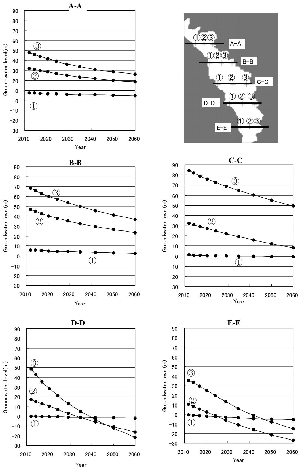
**Figure 1-6 Predicted Groundwater Level (Groundwater Extraction: 740MCM/year)**
