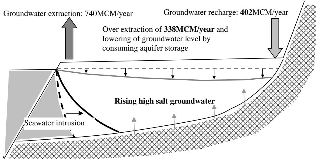
**Figure 1-8 Groundwater Problem by Over-extraction of Groundwater**
