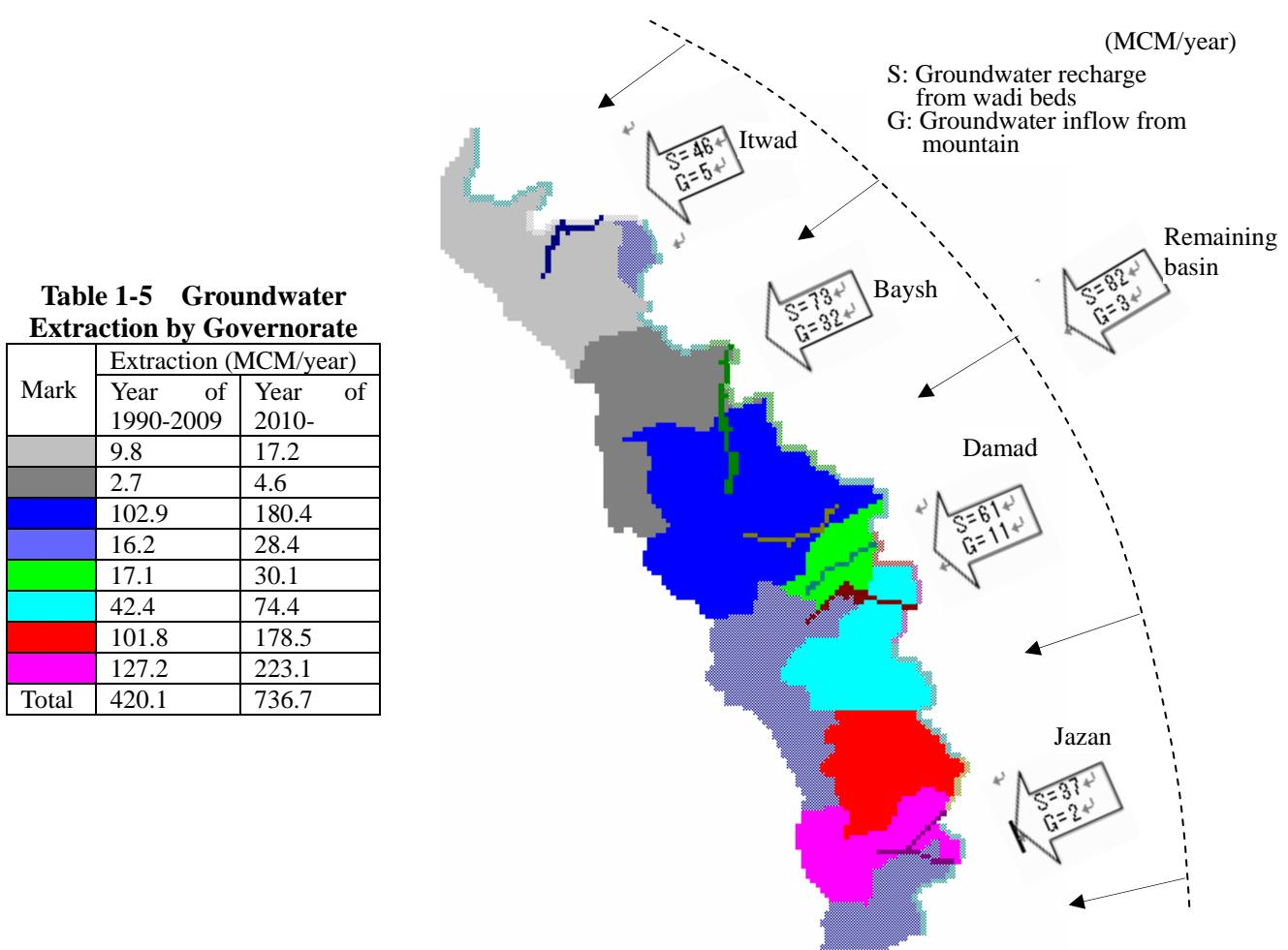
Figure 1-4 Boundary Condition of Simulation
