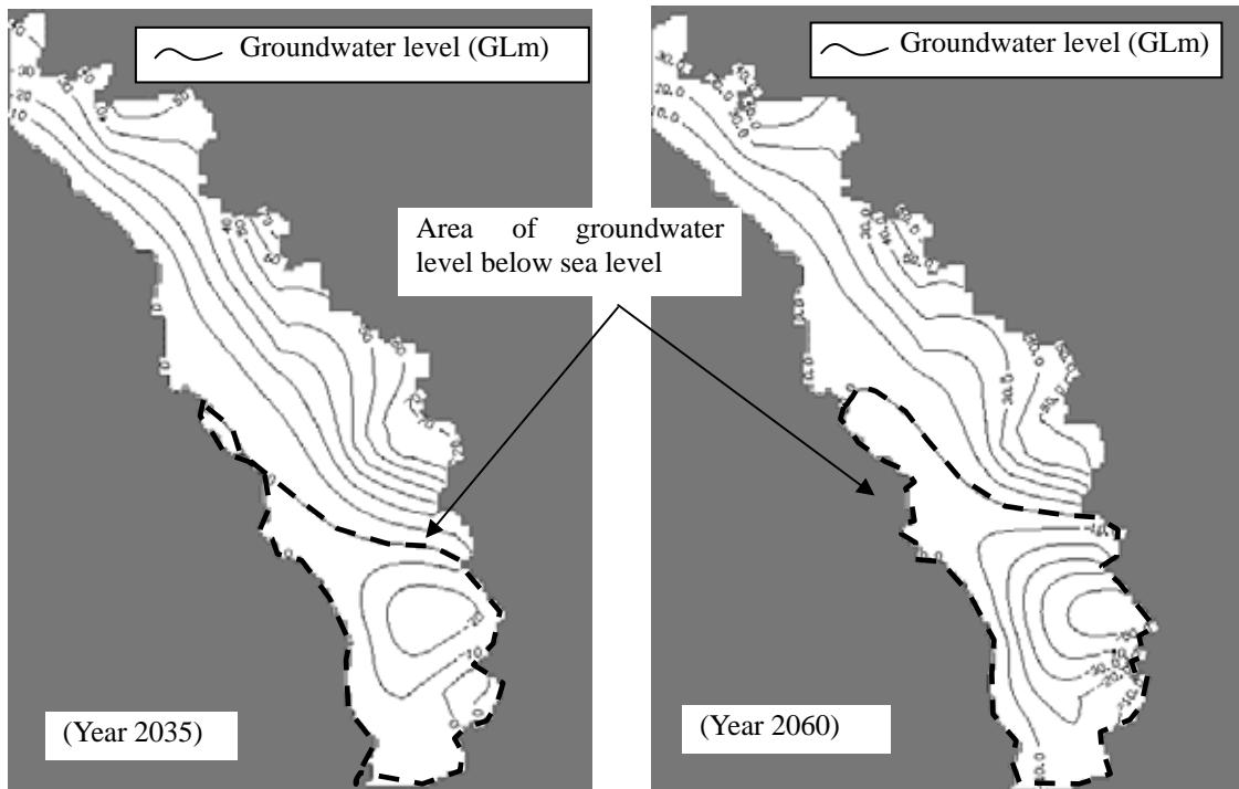
**Figure 1-7 Predicted Area under Seawater Level**
