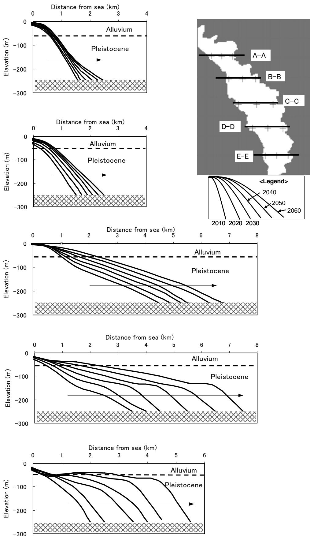
**Figure 1-11 Predicted Location of Interface between Fresh /Seawater (2010-2060)**
