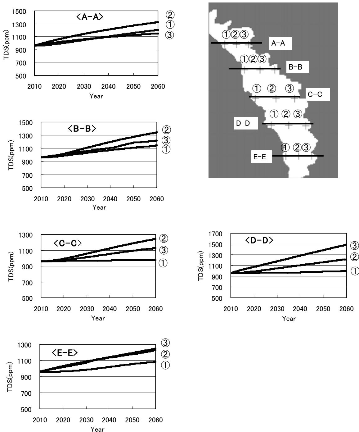
**Figure 1-14 Predicted TDS Concentration of Groundwater by Rising Groundwater from Deep Aquifer**
