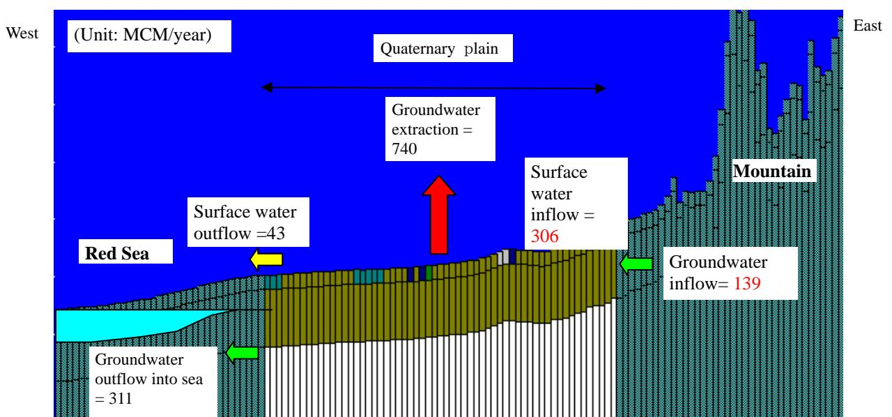
Figure 1-5 Water Balance Given to Model
