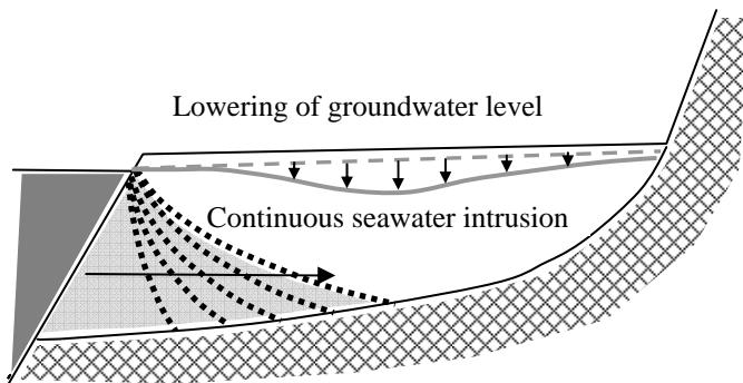
**Figure 1-9 Continuous Seawater Intrusion**
