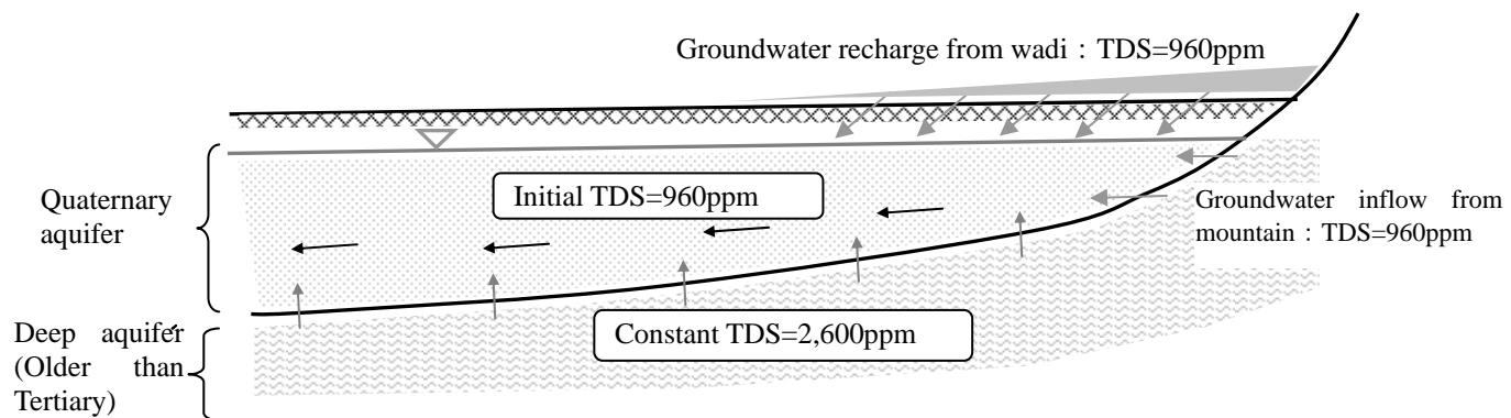
**Figure 1-13 Initial and Constant TDS Concentration of Simulation**
