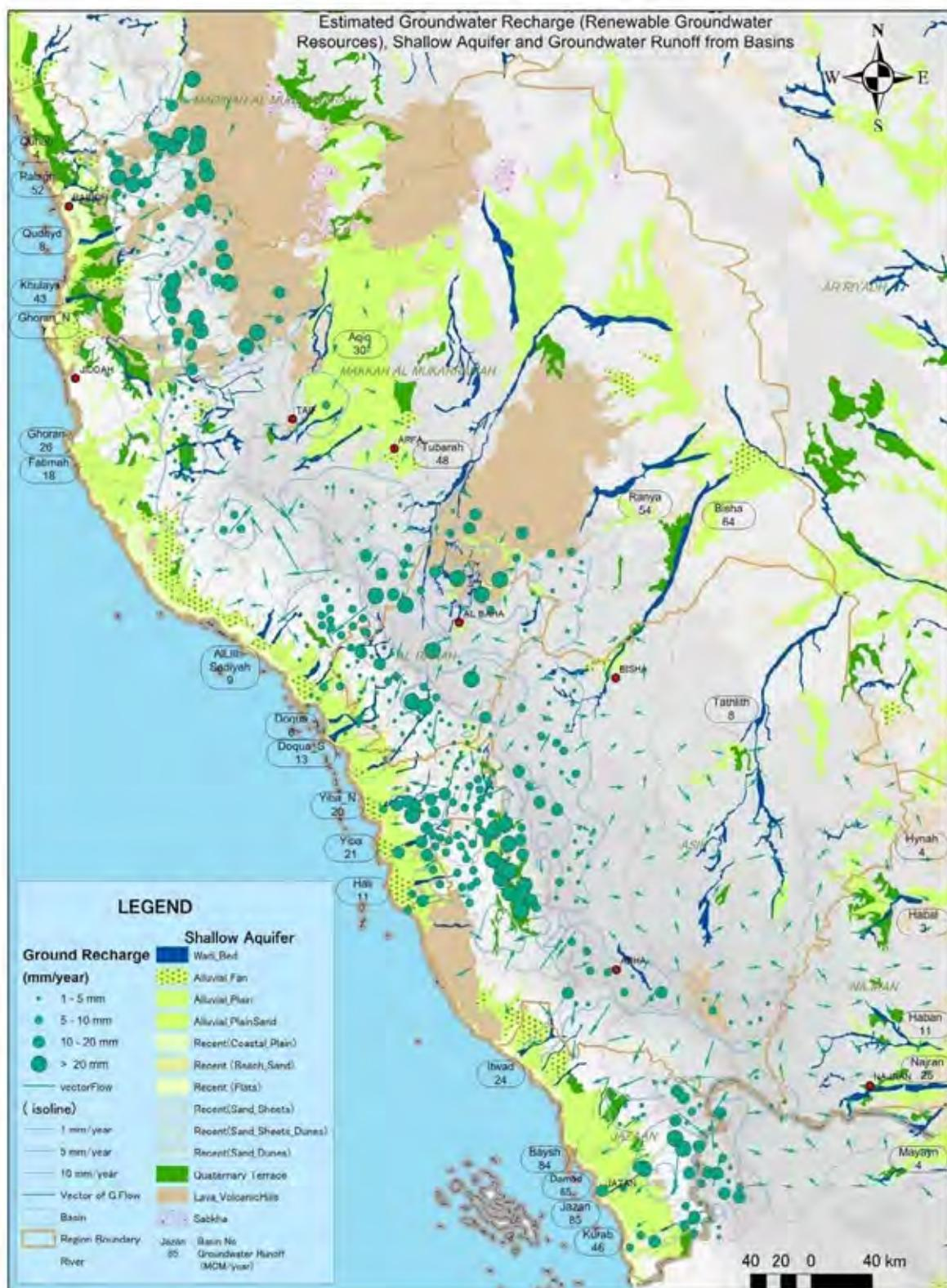
**Figure 4-24 Distribution of Shallow Aquifer and Groundwater Recharge**
