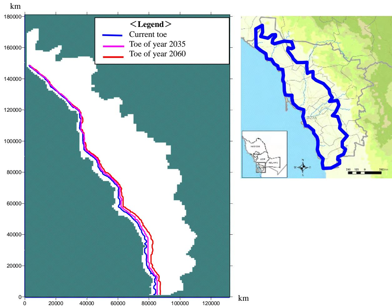
**Figure 1-12 Predicted Area of Seawater Intrusion**
