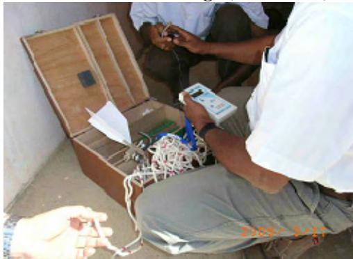
**Photo-11 Portable Current Meter (Habawnah)**
