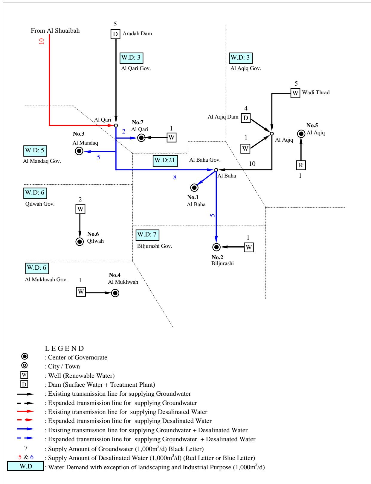
**Figure C.3-1 Water Supply Network in Al Bahá Region (Current)**
