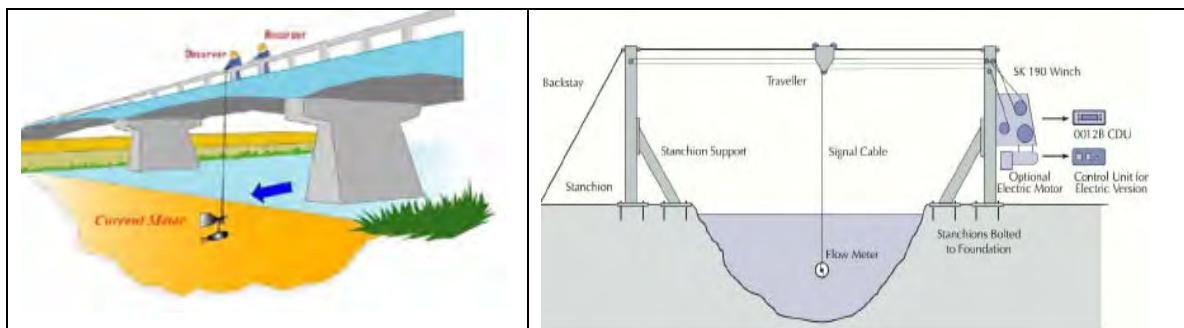
**Figure C.5-10 Current Meter Measuring at Bridge (Left) and Cable-way Type Current Meter (Right)**
