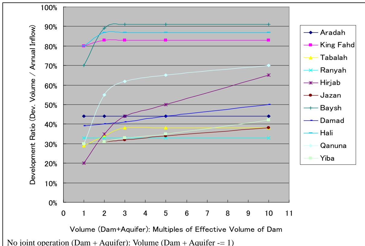
**Figure C.5-3 Variation of Dam Development Volume in Combination with Aquifer**
