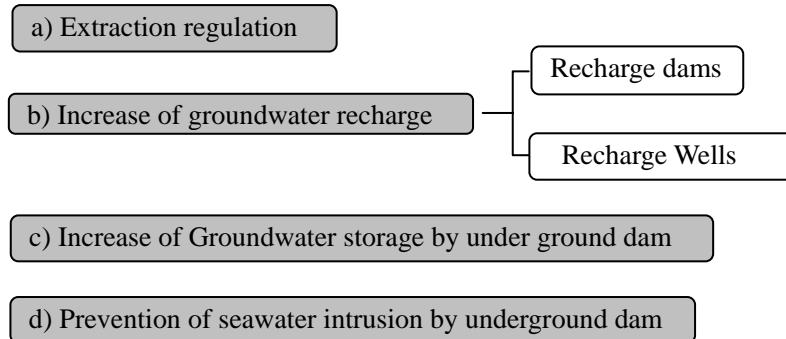
**Figure C.5-14 Method for Groundwater Conservation**
