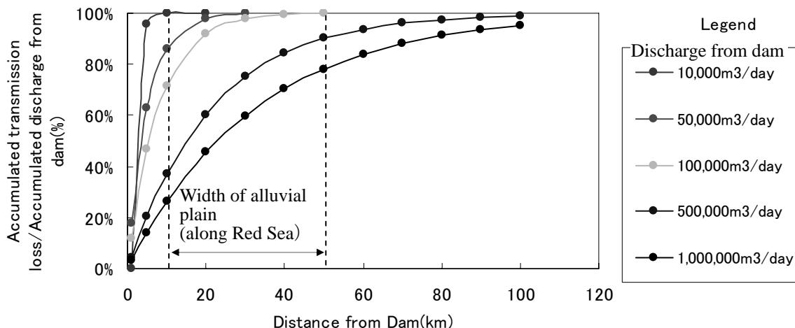
**Figure C.5-6 Example of Transmission Losses and Flow Distance (by Wheater Equation)**
