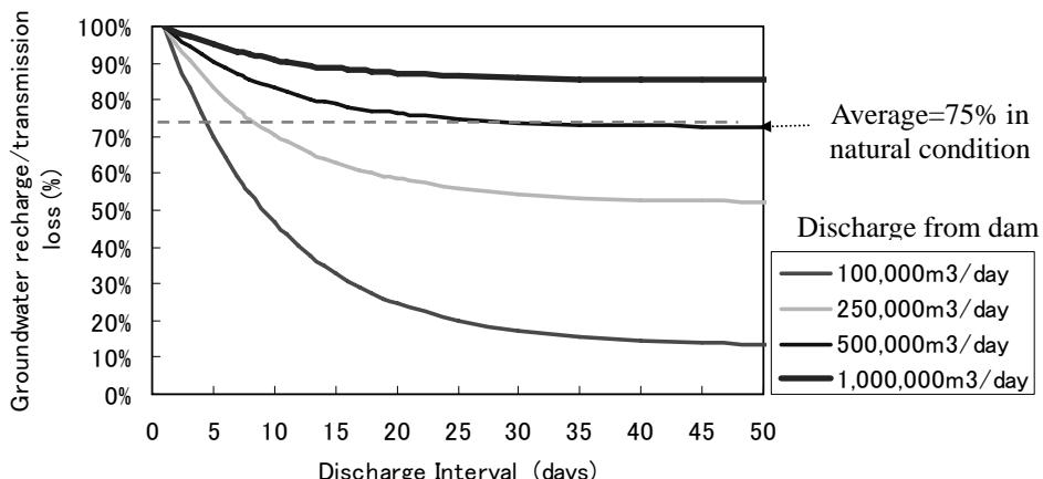
**Figure C.5-7 Relation between Interval of Discharge and Groundwater Recharge**
