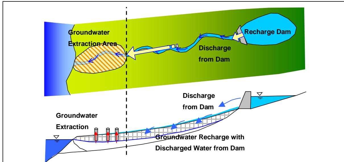
**Figure C.2-3 Groundwater Development by the Recharge Dams**
