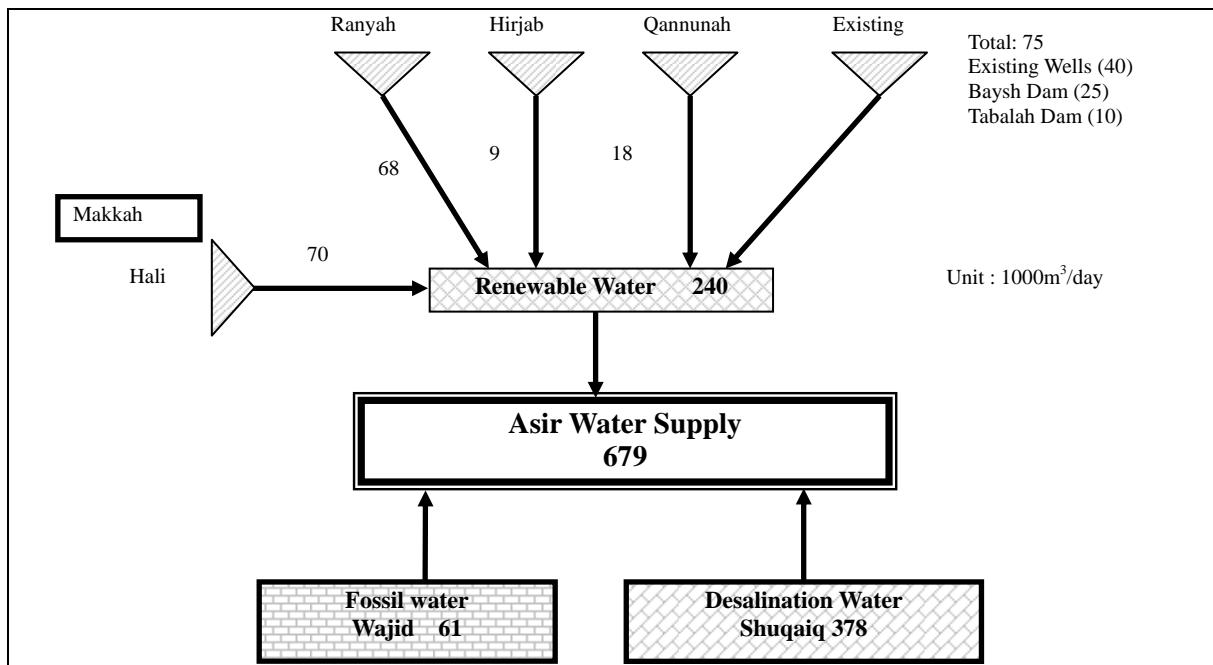
Figure C.3-9 Water Supply Plan and Water Sources in Asir Region (2035)
