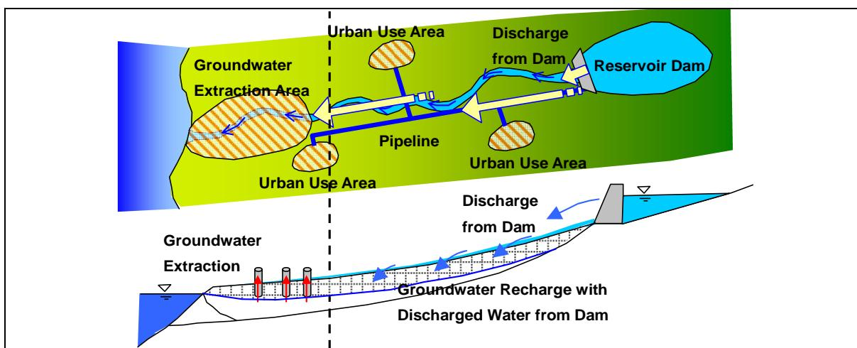
Figure C.2-2 Surface Water & Groundwater Development by Combination with Large Dam and Aquifer
