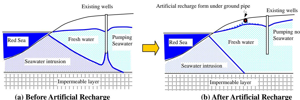
**Figure C.2-10 Measures against Seawater Intrusion by Treated Sewage**
