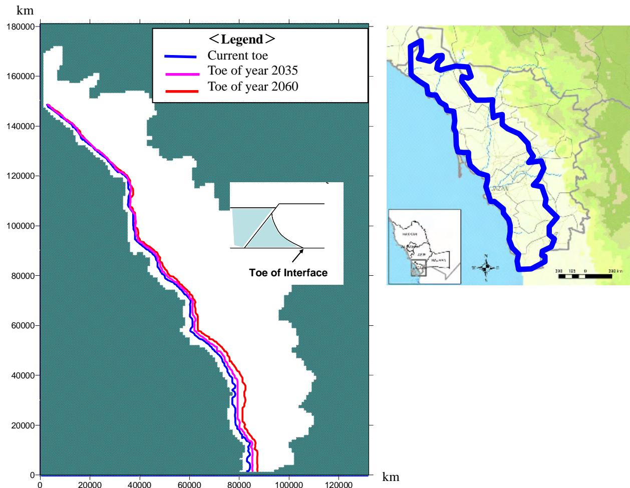
**Figure C.5-11 Predicted Seawater Intrusion by Current Water Extraction (by Study Team)**
