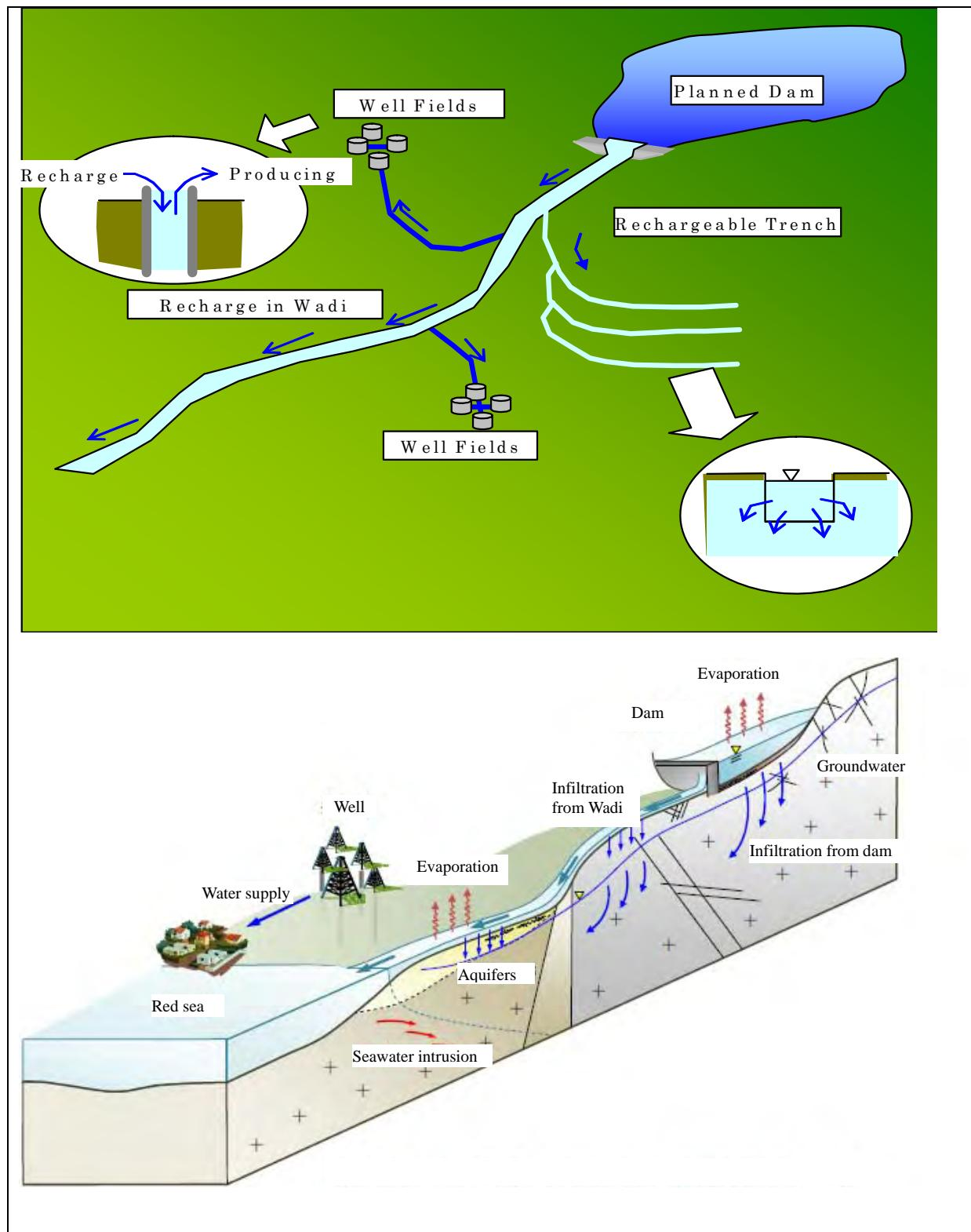
**Figure C.5-2 Recharge of Water from Dam into Aquifer**
