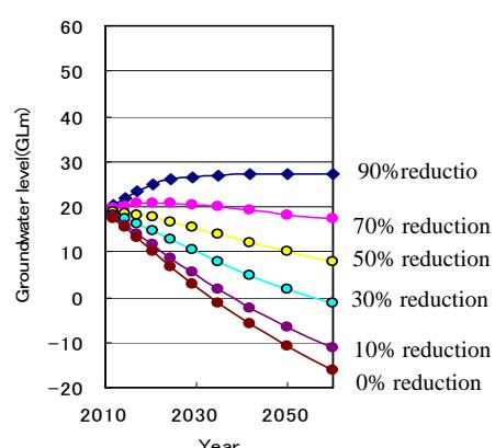
**Figure C 4-4 Recovery of Groundwater Level by Reduction of Pumping Rate**
