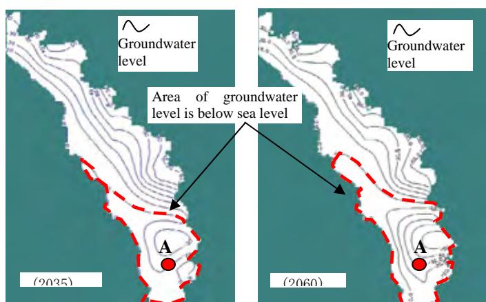
**Figure C 4-3 Predicted Draw Down of Groundwater Level under Current Pumping Rate**
