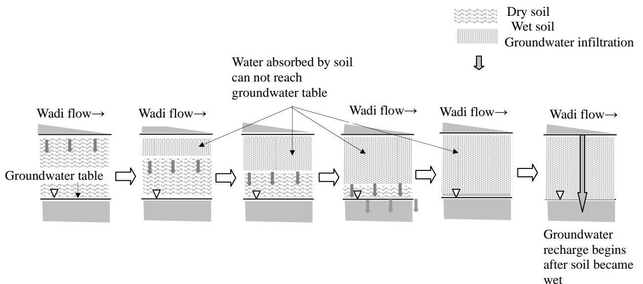
**Figure C.5-5 Groundwater Recharge and Soil Moisture**
