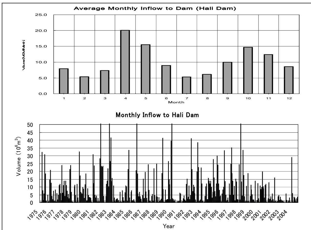
Figure C.2-6 Monthly Discharge Volume to Dam (Hali Dam)
