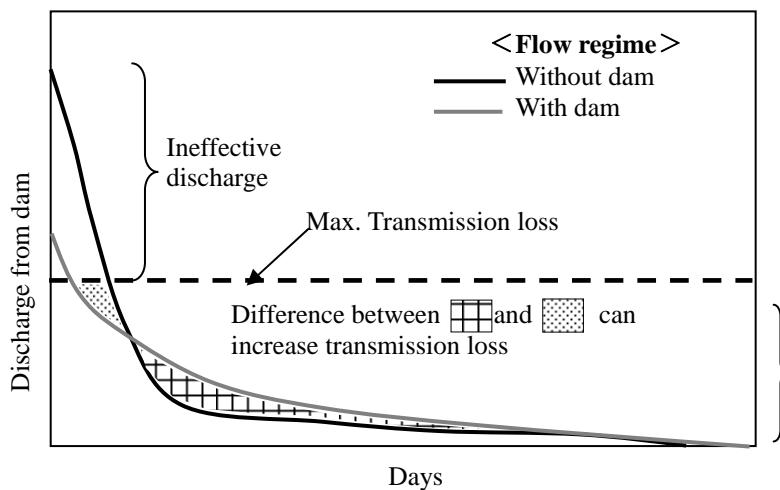
**Figure C.5-8 Improvement of flow Regime and Increase of Transmission Losses**
