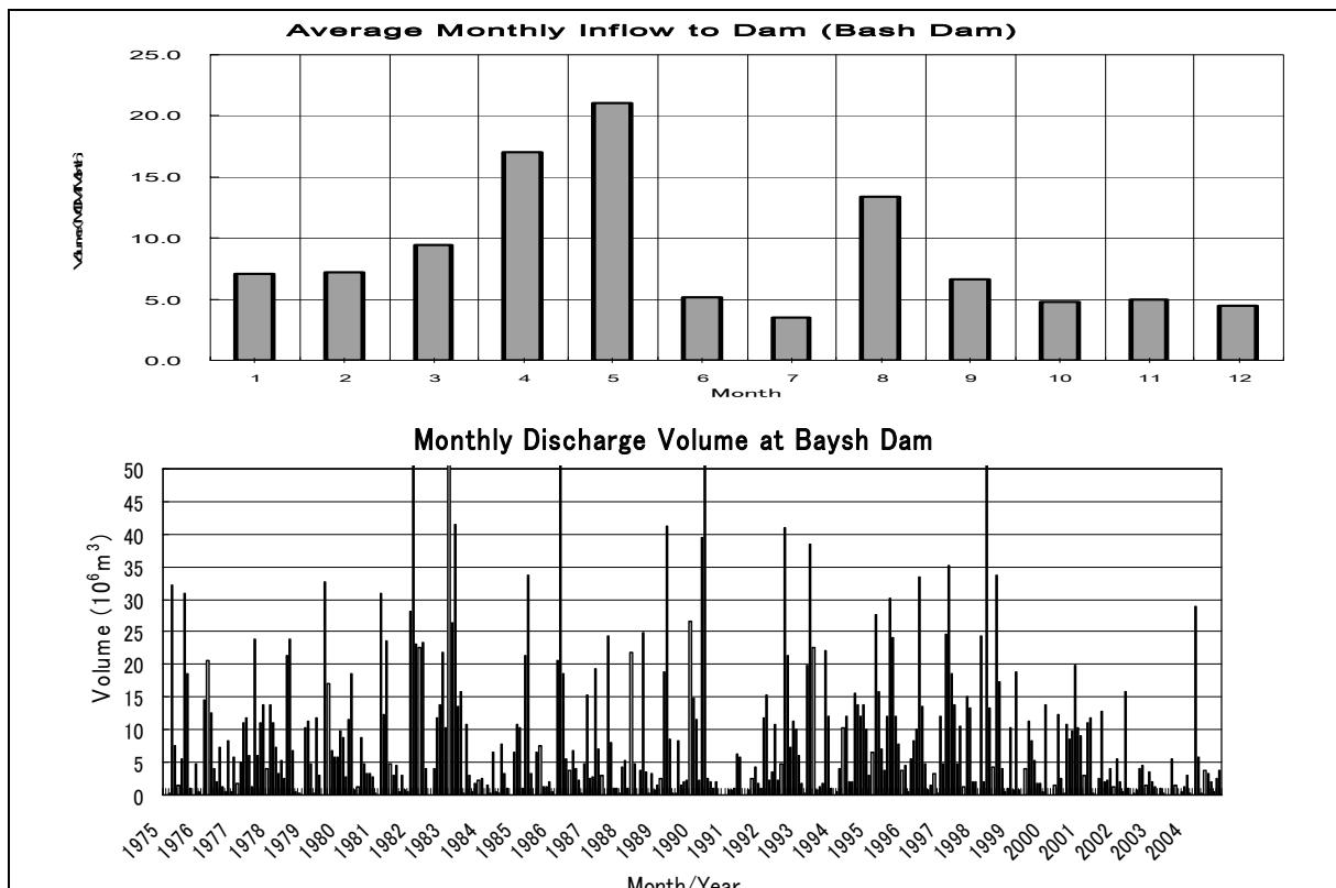
Figure C.2-5 Monthly Discharge Volume to Dam (Baysh Dam)
