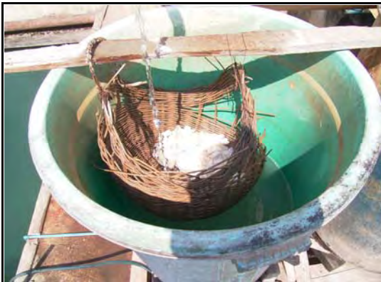
Photo 4-3 Solid alum in bamboo basket. They pour water to dissolve it.
