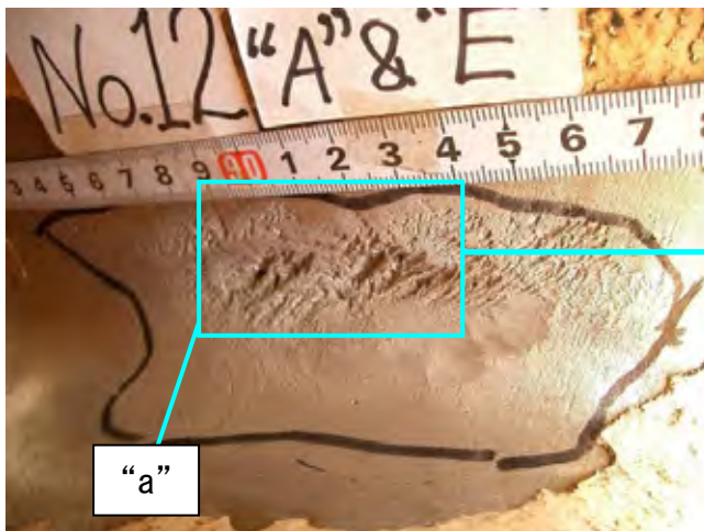
Cavitation at Inlet Side
