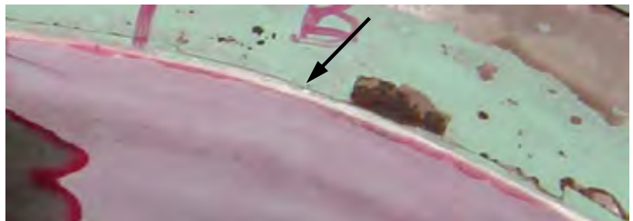
Babbitt Metal has been detached from the Bearing Support
