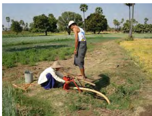
Treadle pump provided to Kan Ma village, irrigating onion field.
