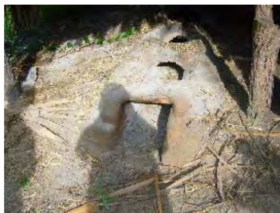
An improved stove for Jaggery production. Though it is efficient in energy consumption, it has not been diffused due to the cost.
