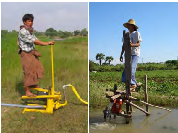
Two Types Treadle Pumps: Left one can push irrigation water up to over 13m while right one only 5-6 m but very simple structure which can be produced even in their locality.
