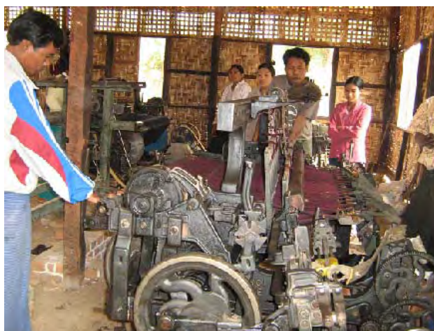
Engine driven weaving machine installed in Ma Gyi Sauk village, which needed periodical repair, adjustment, and maintenance.
