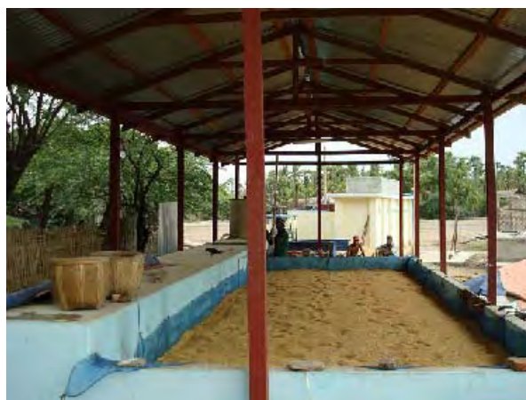
Paddy dryer established in Legaing village as a part of pilot project under cottage sector. This can dry 200 baskets of paddy at a time.
