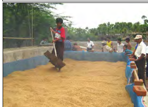
Photo 2: Paddy dryer (Legaing Village) using rice husk. They are now drying pre-monsoon paddy which is usually harvested during the onset of rainy season, thereby needing drying.
