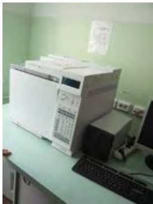
【No.20】 Nov. 6, 2009 Petropavlovsk Hygiene and epidemiology inspection center Gas Chromatograph for pesticide residue analysis
