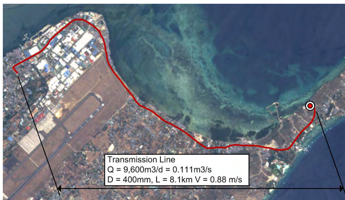
Figure III-22 Transmission Route from Desalination Plant
