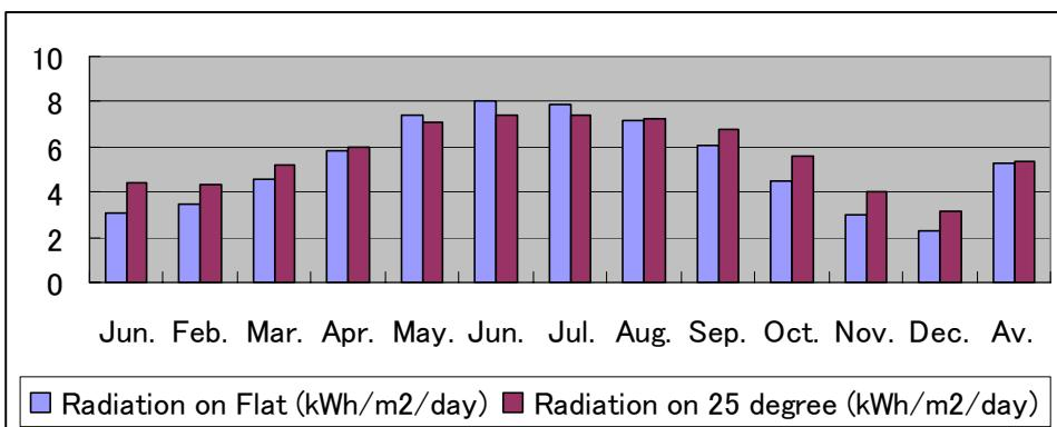
**Figure 2-2 Monthly Average Radiation (PV panel setting angle: 25 degrees)**
