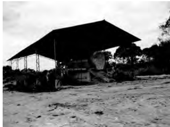
The rotary sieving machine for composting located at the Manaus municipal landfill.
