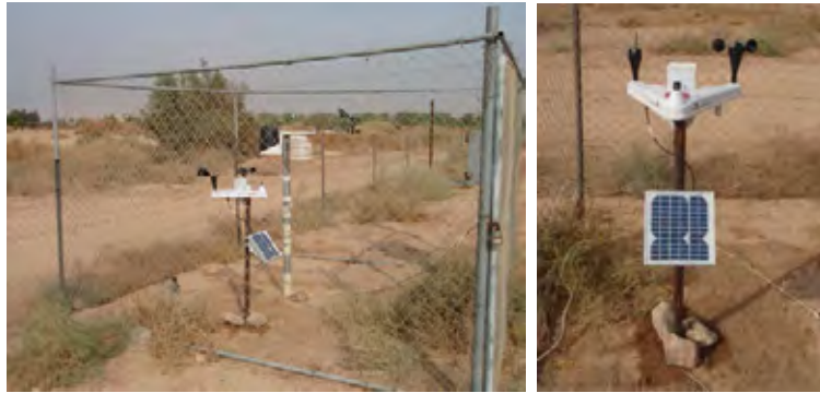
Photo Left : The device (left) used for measuring solar radiation and temperature
