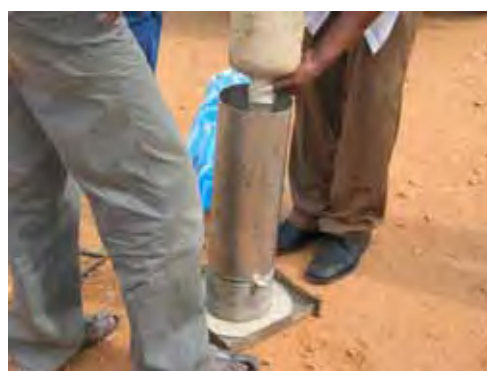
Figure 24.4.3-4 Sand Cone Replacement Test at Site
