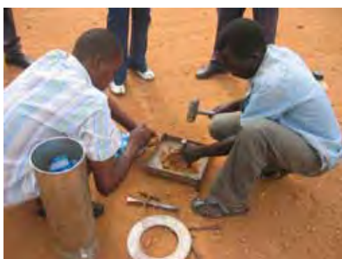
Figure 24.4.3-4 Sand Cone Replacement Test at Site
