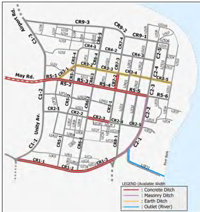
Figure 17.2.3-3 Present Drainage Type (as of May 2009)
