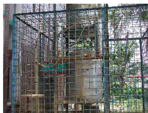
Figure 3-12-3 “SIDKO” (which is one of arsenic removal equipment for community use)
