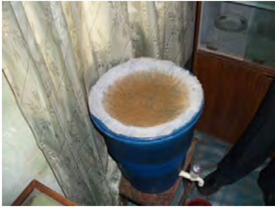
[Arsenic removal facility in DPHE office in Muradnagar] Filter media has not been changed.
