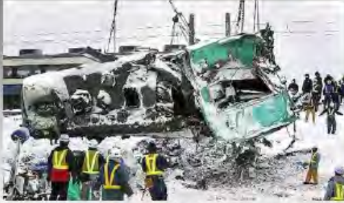
Derailment by Strong Wind of Uetsu Line, 2005
