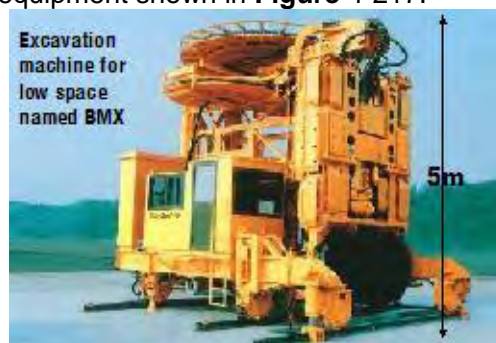
Figure 4-217 Special Equipment, BMX, for Construction of Diaphragm Wall
