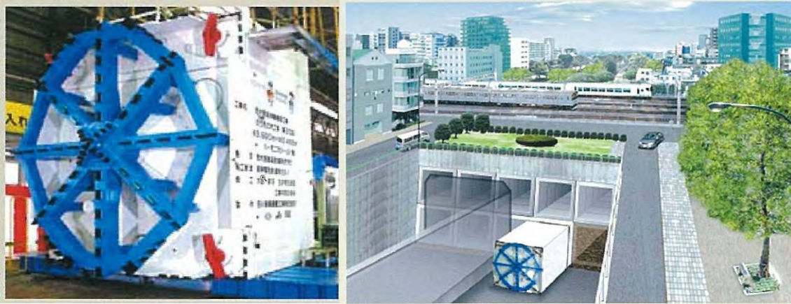
Figure 4-19 Photo of Multi Box Jacking Machine and Image of Construction
