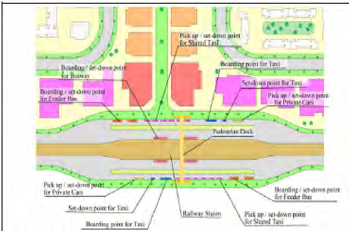
Figure 2-57 Plan Arrangement of “Pick-up and Set-down” Facilities for Feeder Transport at Ordinary Stations
