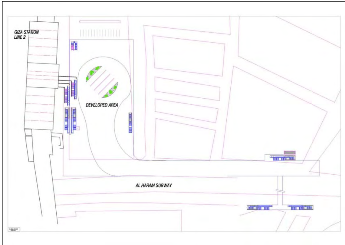
Figure 2-56 Concept Drawing of El Giza Station, Showing the Layout of Above-ground “Park and Ride” and Modal Interchange Facilities
