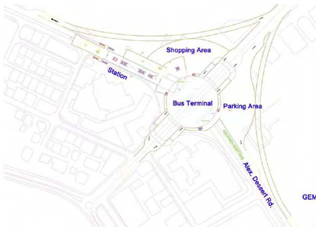
Figure 2-55 Concept drawing of El Remayah Station, showing the layout of Underground “park and ride” and modal interchange facilities
