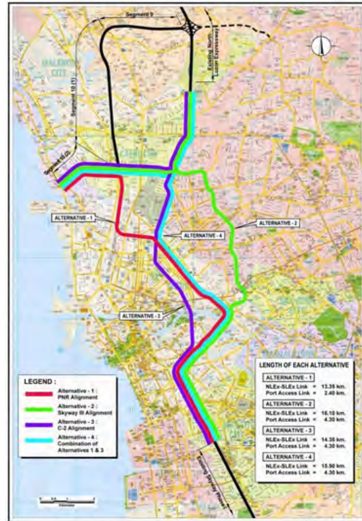
FIGURE 14.1.1-2 NLEX-SLEX LINK EXPRESSWAY ALTERNATIVES: CASE-2
