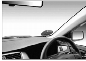
Figure 5.4.5 ETC at Toll-island (1-piece)
