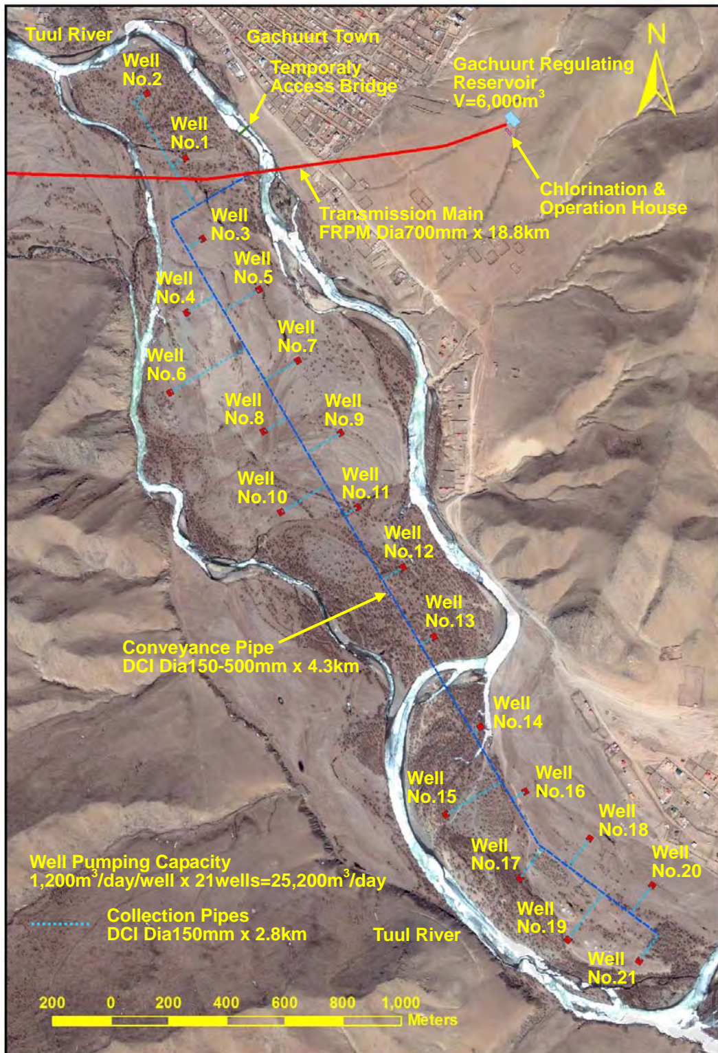
Figure 2-2.9 The Alignment of Collection and Conveyance Pipes
