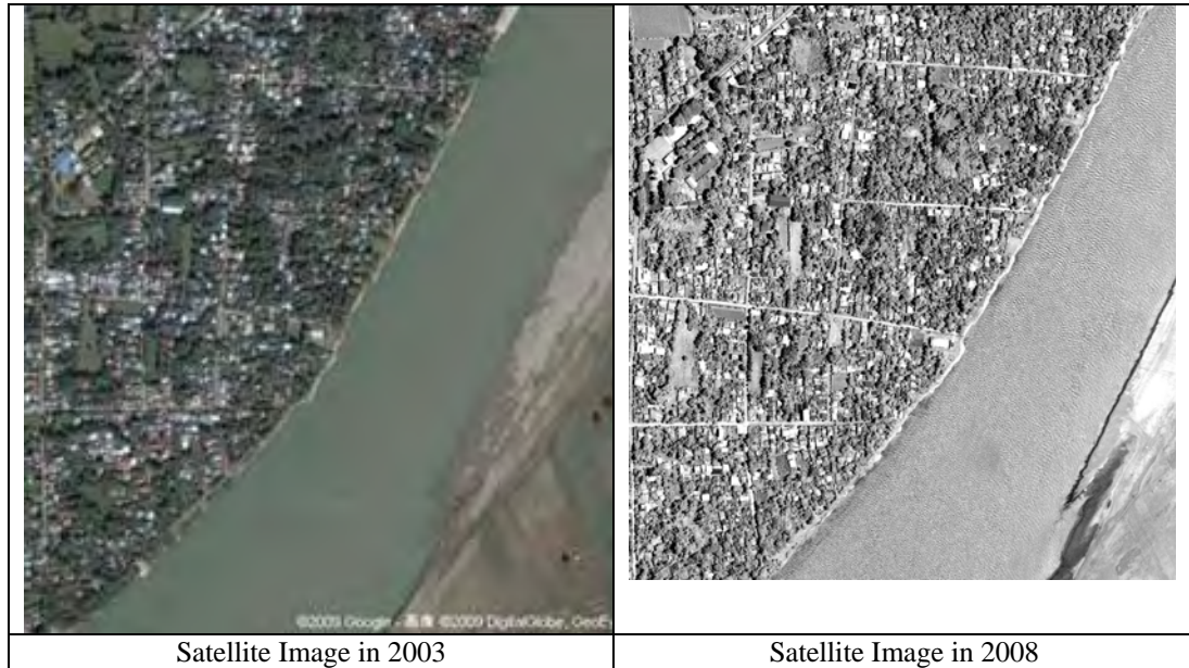
Figure R 7.3 Comparative Photos for Progress of Erosion at Cataggaman
