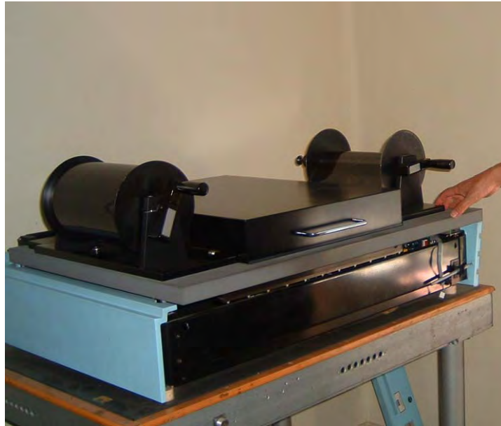
Figure 2.15 Scanning of a roll film by “Vexcel Ultrascan 5000”
