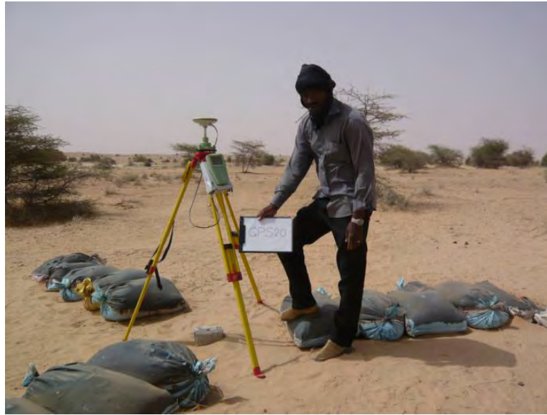
Figure 2.8 GPS observation at a point (GPS20)
