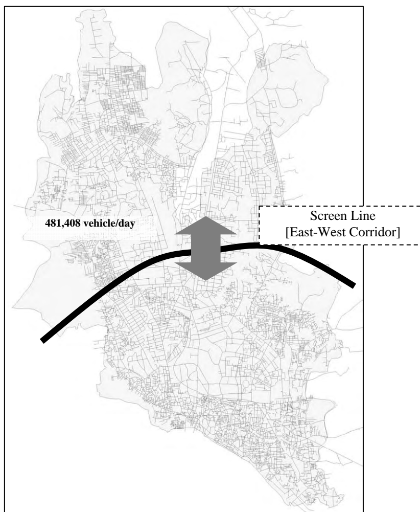
Figure 3.3-2 Main Screen line Survey Location
