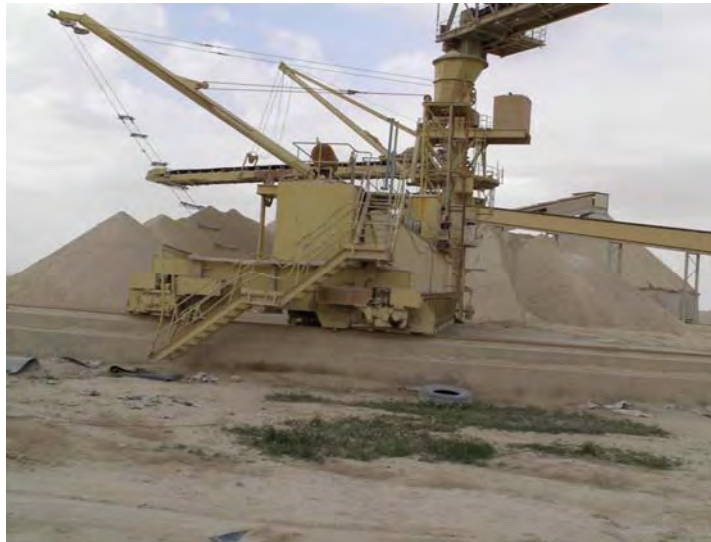
Figure 6.2-6: Stacker and Reclaimer
