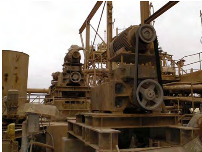
Figure 6.2-14: Gear Box and Motors on Phosphoric Acid Reactor
