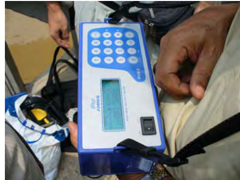
AMNIS PVM-3 (Type II) portable current meter
