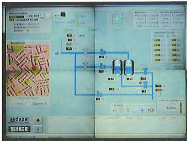
Example of panel display for SCADA
