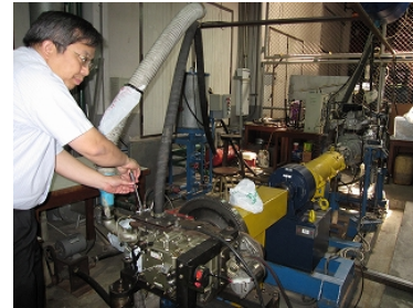
Dynamometer with endoscope of Mechanical Engineering Department, Faculty of Engineering
