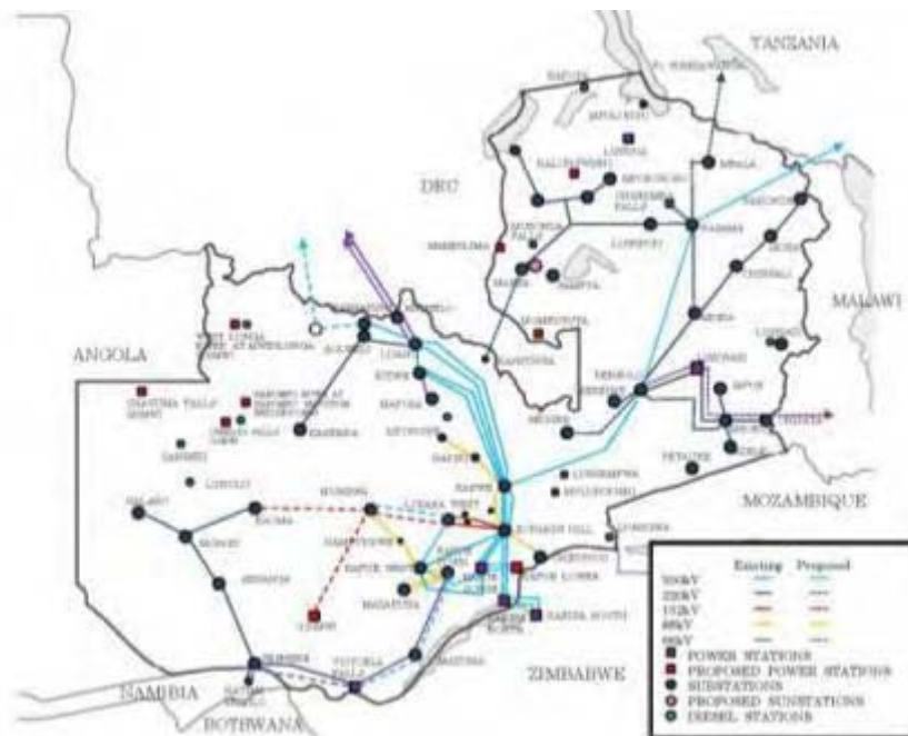
Figure 8.1 Transmission system in Zambia
