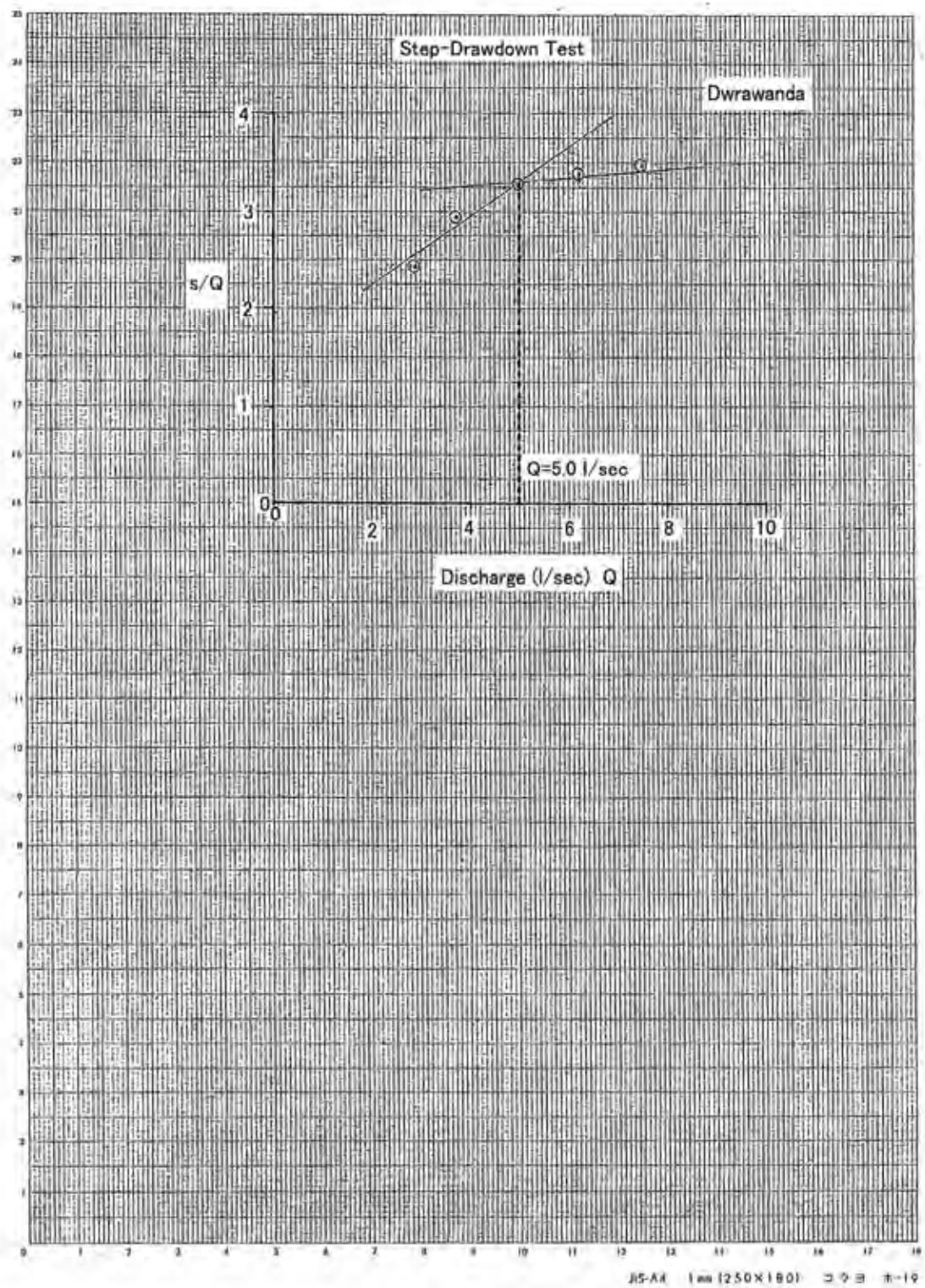
Fig 13 Step drawdown test in Derawanda
