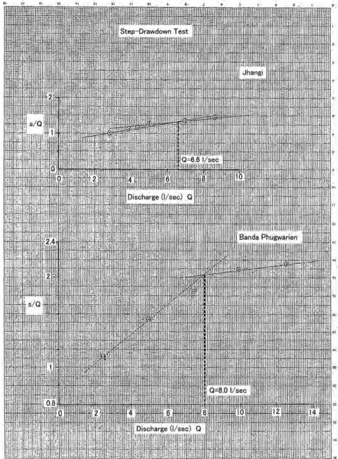
Fig 13 Step drawdown test in Jhangi and Banda Phugwarian
