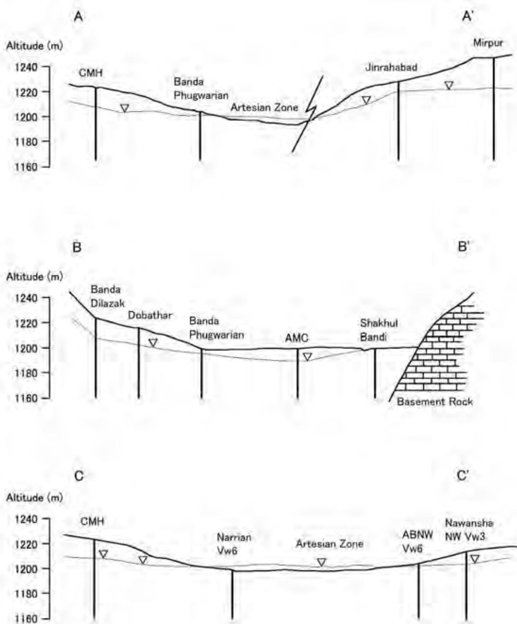
Fig. 6 Profile of Static Water Level
