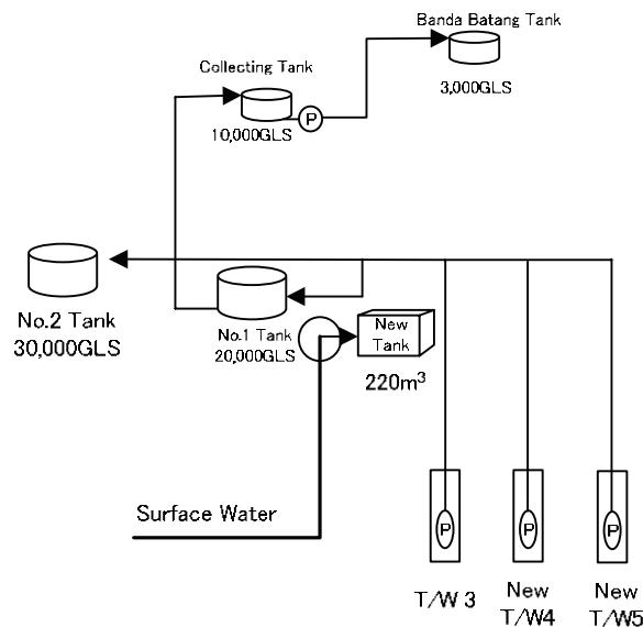
**Figure 2-2-10 Abbottabad District Water Supply Scheme (Derawanda System)**
