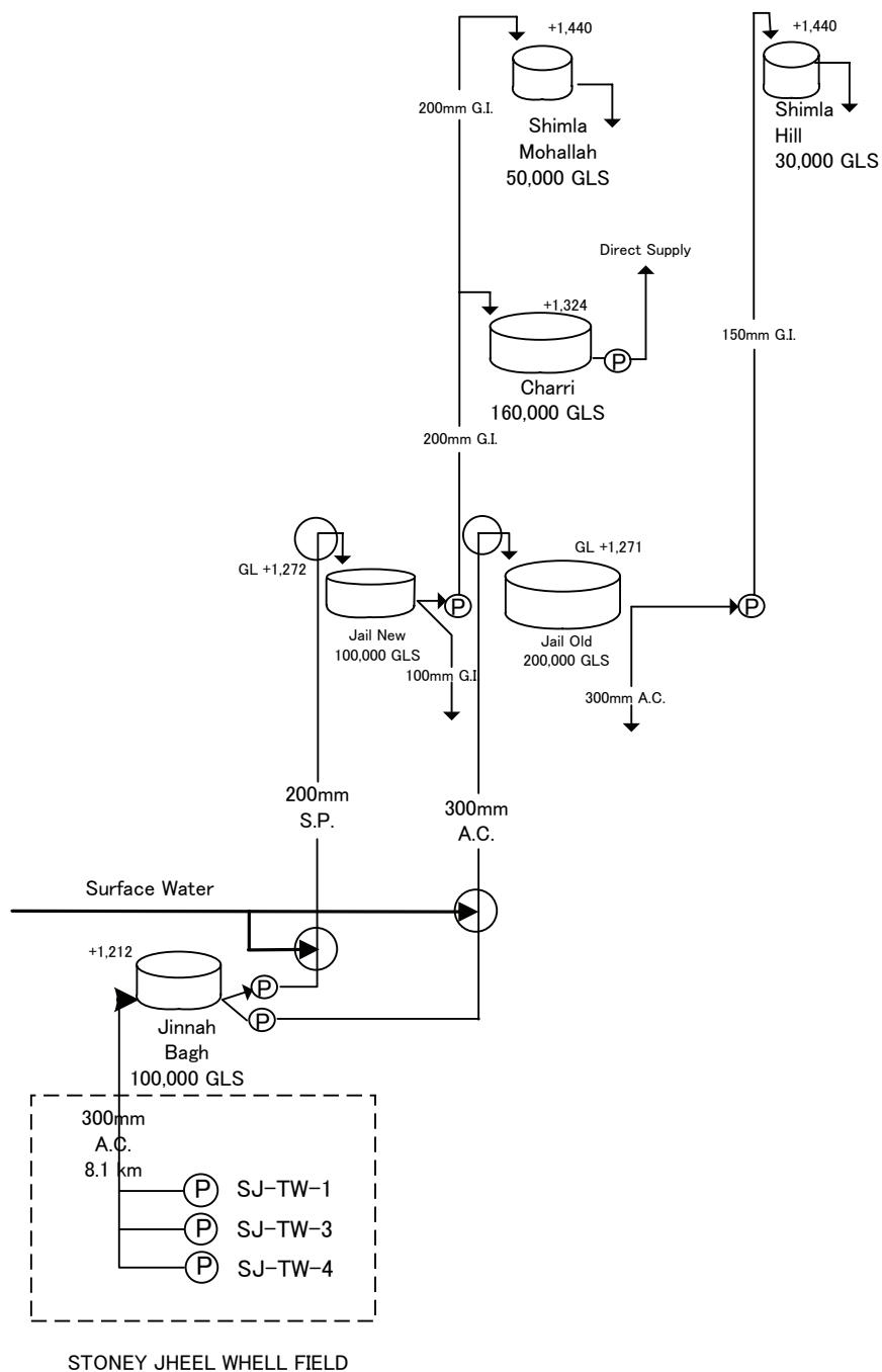
**Figure 2-2-5 Abbottabad City Water Supply Scheme (Jinnah System)**
