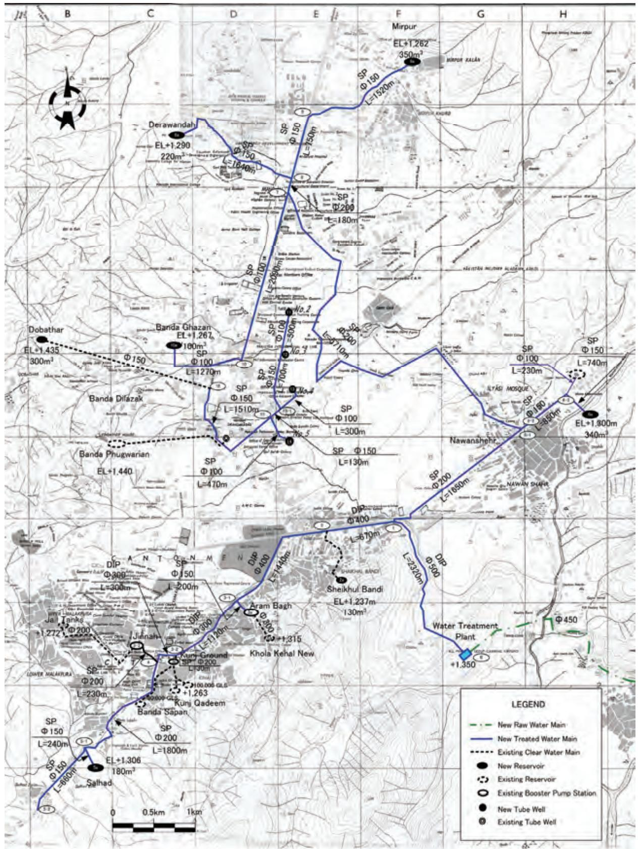
Figure 2-2-2 Location of Treated Water Transmission Main, Tubewells and Reservoirs
