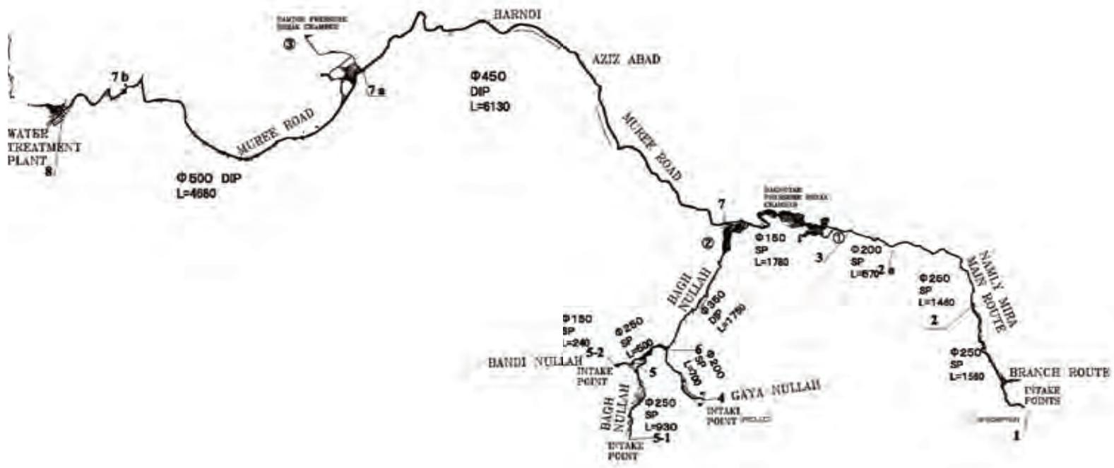
Figure 2-2-1 Location of Intakes, Raw Water Transmission Mains, Pressure Releaseing Chambers, Water Treatment Plant
