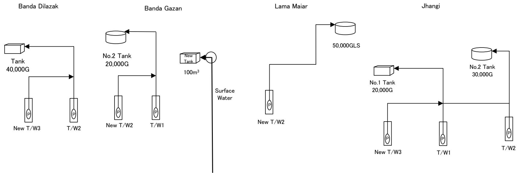
**Figure 2-2-11 Abbottabad District Water Supply Scheme at Jhangi UC.**
