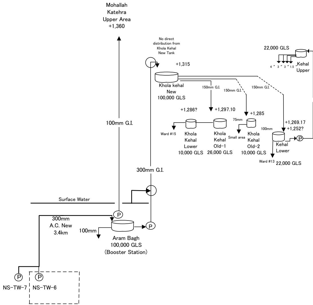
**Figure 2-2-3 Abbottabad City Water Supply Scheme (Aram Bagh System)**
