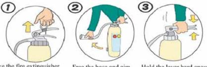
Take the fire extinguisher close to the fire, and then pull the safety pin with a finger to upright.
