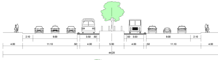
Figure 5.4-3 Existing and Planned Cross Sections on Av. Almirante Barroso (2)
