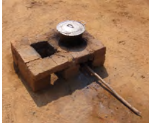
Improved stove made by a participant of workshop. (The bottom of pot can be burned because of square hole)
