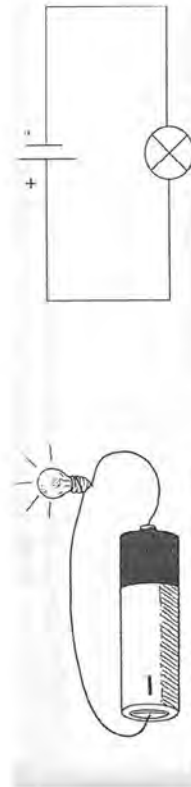
Figure 8.12 A simple electric circuit
