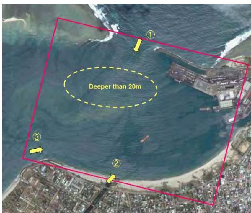
Figure 6-3-7 Topographical changes in the north beach and the Port Beach
