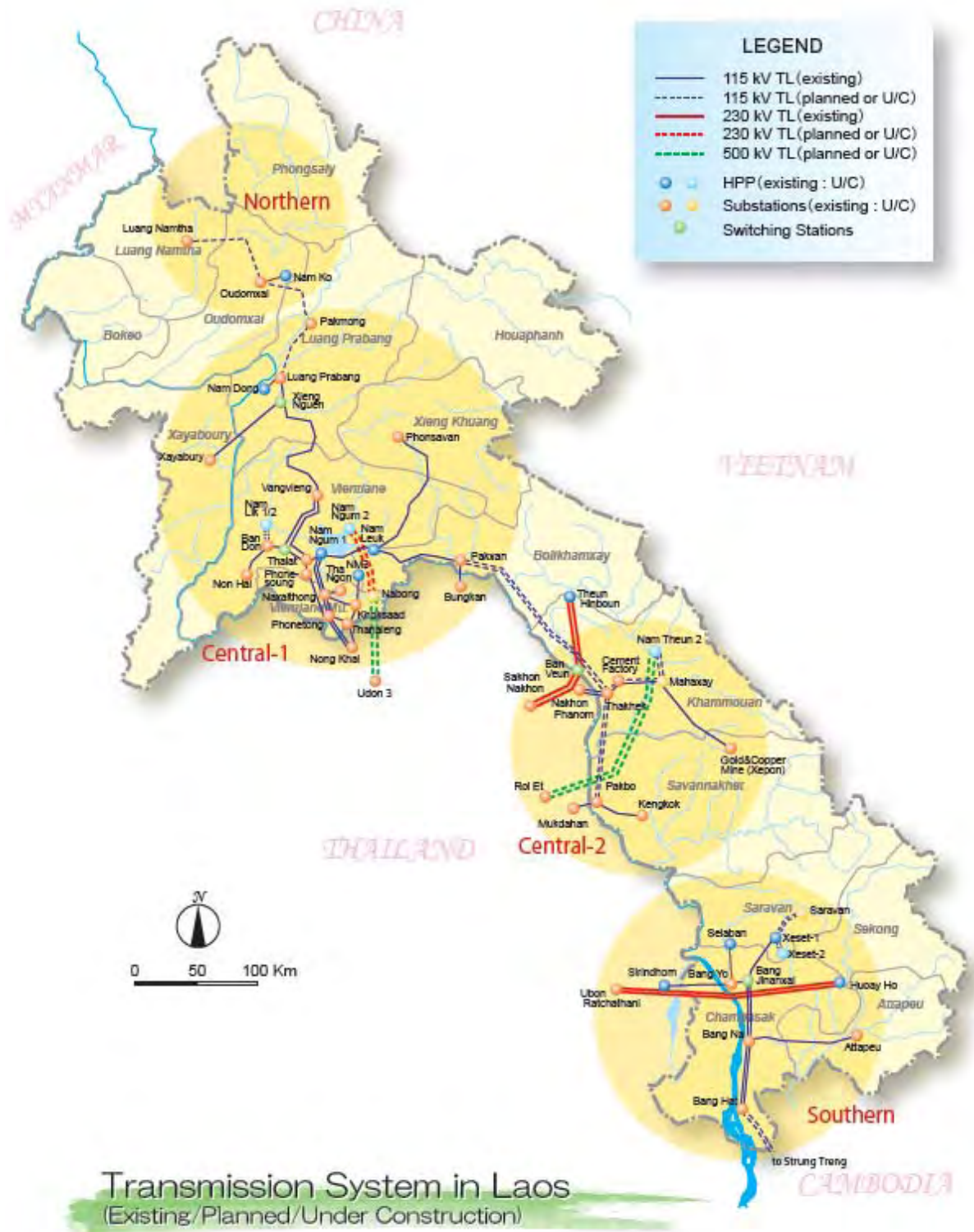
Figure 1-1 Transmission System in Lao PDR (source: Long-term Power Development Plan 2007-2016, EDL et al 2009)
