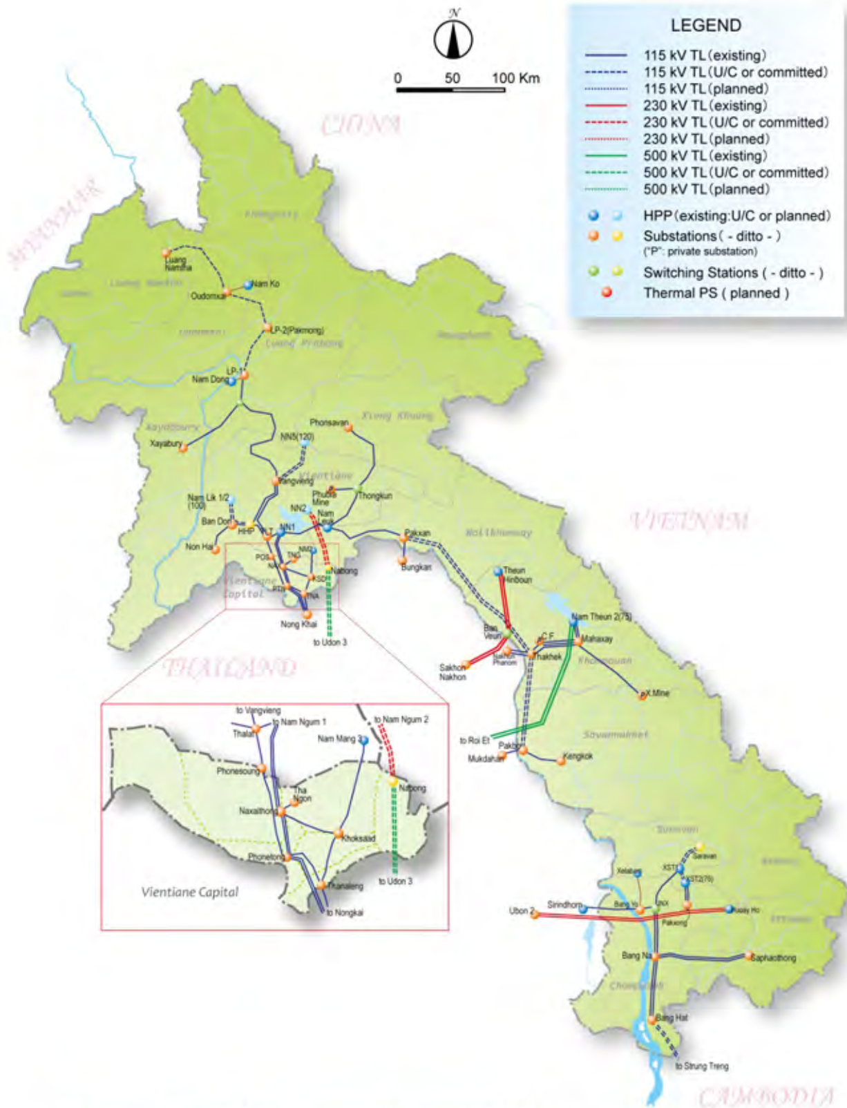
Existing Laos Transmission System in 2009
