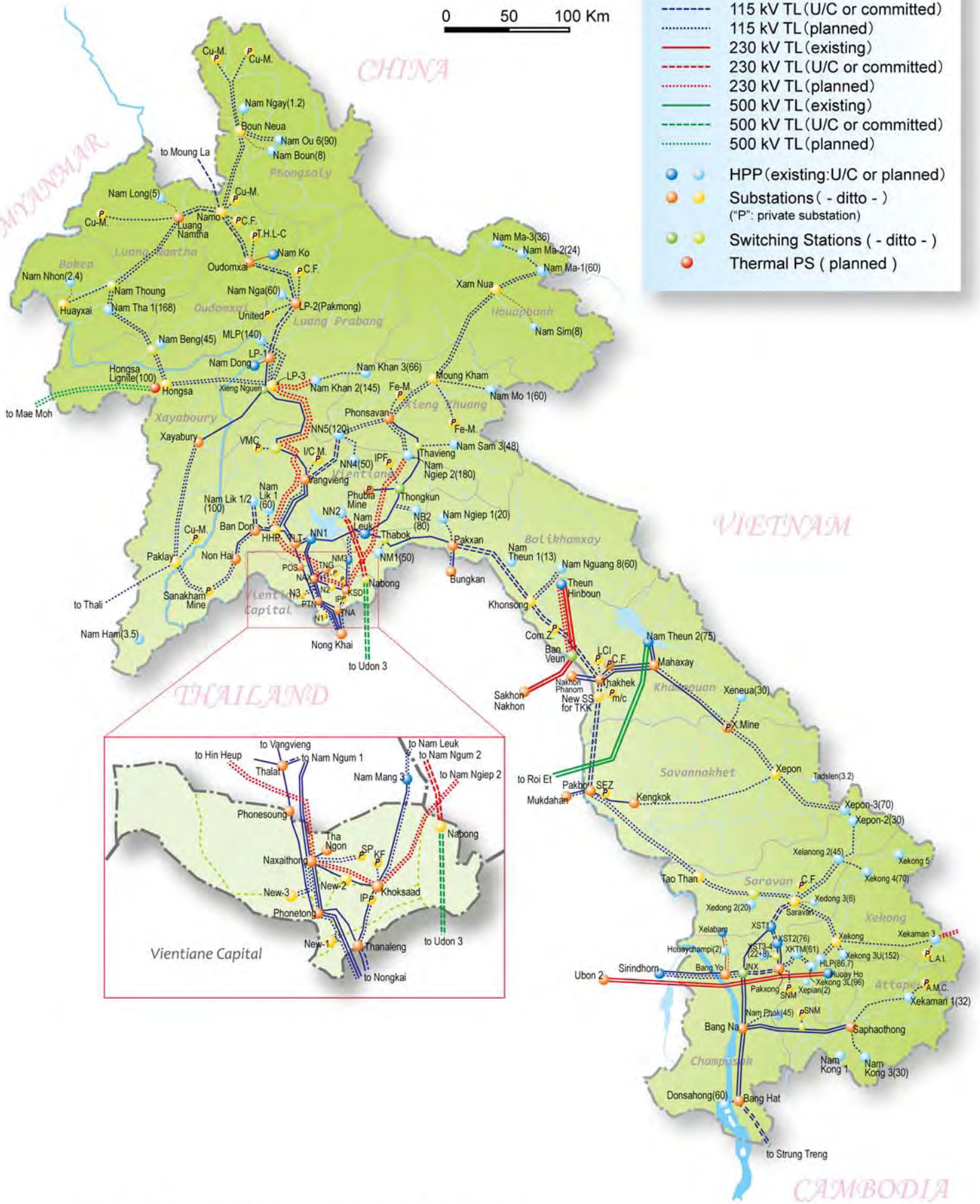
Laos Transmission System in 2020
