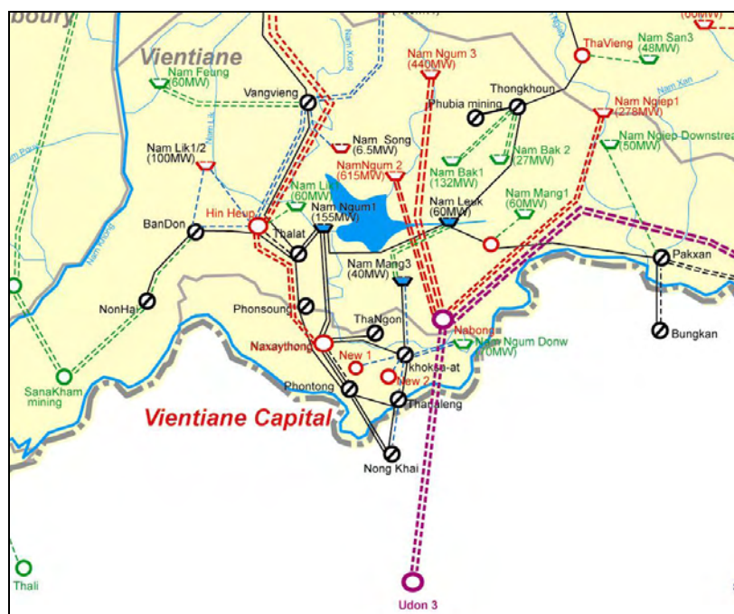
Figure 4.11 System Configuration of C1 Area, Vientiane Municipality, 2016
