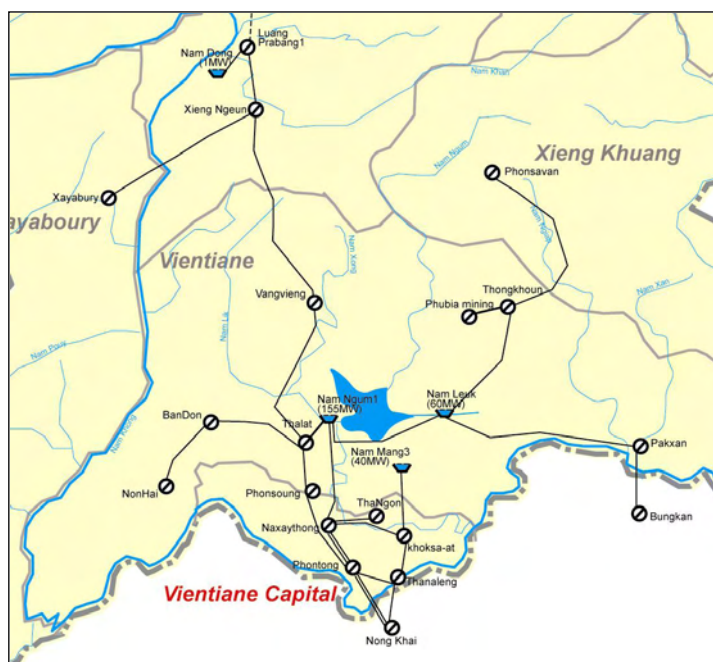
Figure 4.10 System Configuration of C1 Area, Vientiane Municipality, 2009
