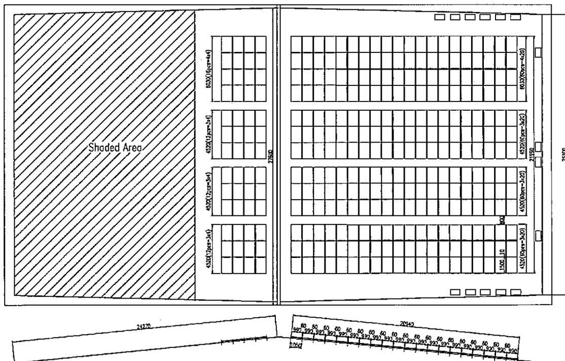
Figure 3-1 Sample PV panel layout (Series Number = 12 pcs)
