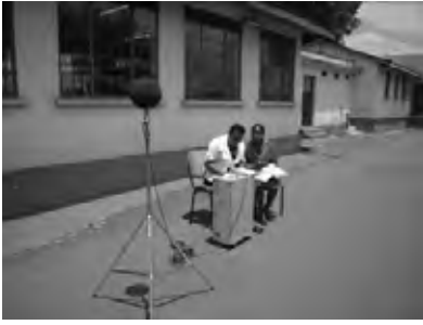
Overview of Noise Equipment (all weather type). At least 2 persons are necessary for this survey
