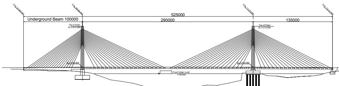
**Figure 6.14 Profile of the New Nile Bridge**
