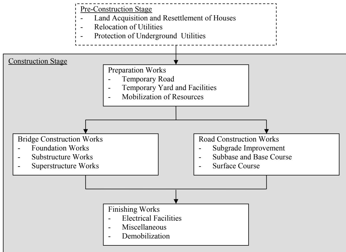
Figure 7.1 Construction Method of the Proposed Nile Bridge
