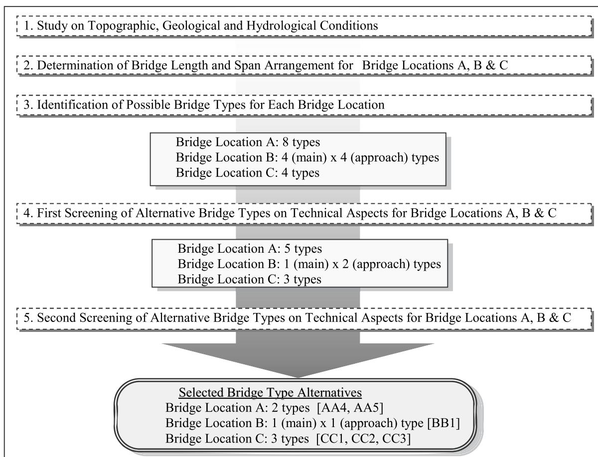
**Figure 3.7 Flow Chart for Selecting Optimum Bridge Types for Bridge Locations A, B & C**
