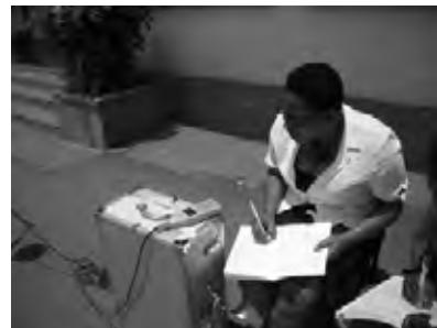
Surveyor 1 writes measured noise level on the survey sheet
