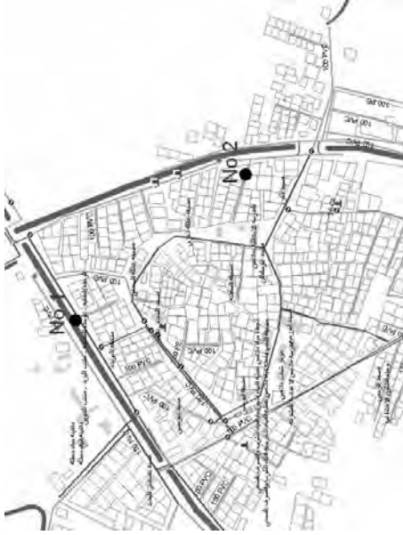
Figure 8-3 Location of detected leaks in Minia Alqamah Markz Area-3
